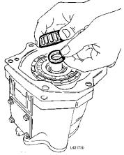
Figure 5 Removing bearing and spacer washer
