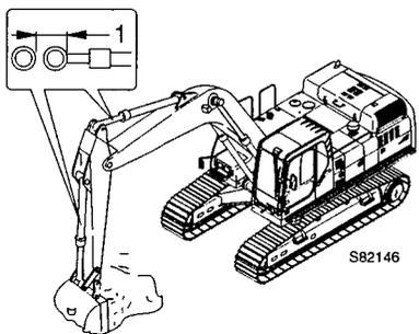
**Do not extend the hydraulic cylinder to its end of stroke**
