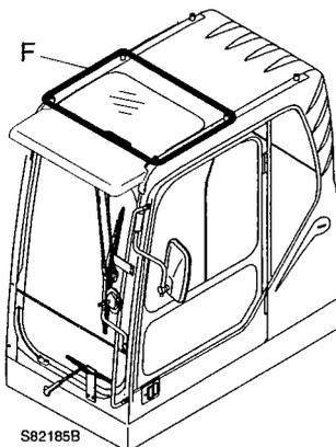
F Tightening torque: 10 kg·m (22.5 lb·ft), Thickness 2
