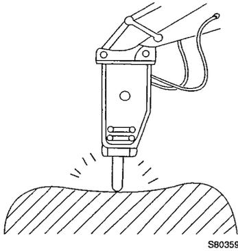
Press the chisel firmly against the surface so idle striking is avoided.
