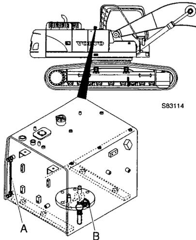
Clean fuel is essential for trouble-free running of the diesel engine. The fuel tank holds **350 liters (92.5US gal)**.
