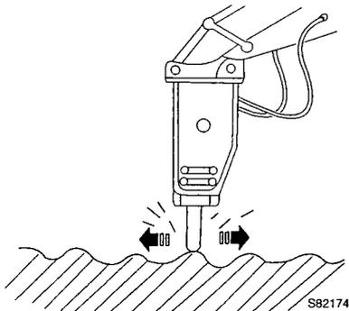
Do not move the chisel while it is striking a blow.
