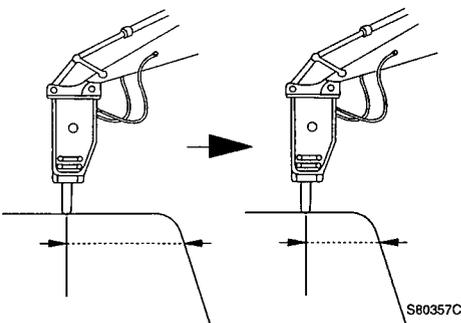
The striking direction of chisel and the direction of breaker body are deviate slightly. Therefore, adjust the bucket cylinder so that the direction of body and chisel is always the same.
