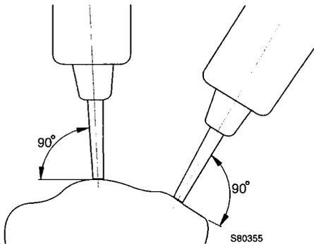
When striking, press the chisel firmly onto the surface, and lift the frame about 5 cm. Never raise the machine unnecessarily high.
