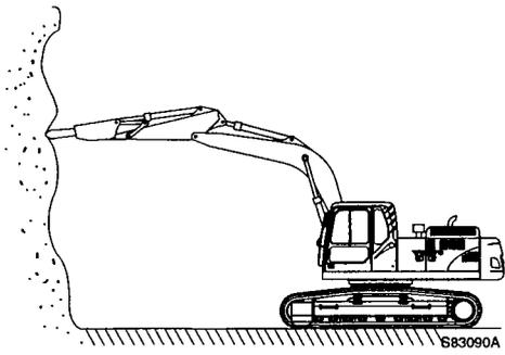
Do not strike horizontally, or in an upward direction.
