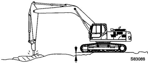
If the surface is struck repeatedly but it does not break within 1 minute, move the chisel nearer one end and strike again.
