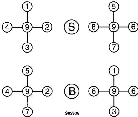
The machine control pattern can easily be changed to the ISO system or to the backhoe loader hydraulic system by changing position of pattern change valve (if fitted). Use the following procedure to change the position of the pattern change valve (Machine standard position is ISO pattern type (S)).
