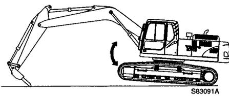
Do not raise the machine by extending the bucket cylinder to maximum.
