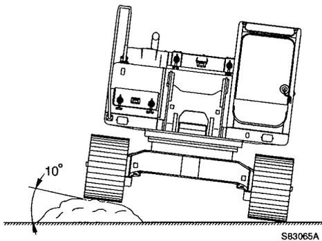
In case of traveling on uneven ground, operate the machine so as not to lean on one side more than 10°.
