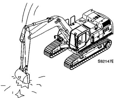
**Do not work by slamming the bucket into the ground**
