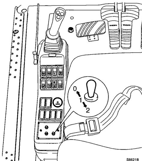
**26 Emergency engine speed control switch**
