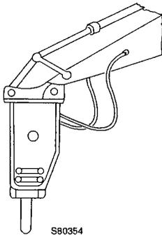
Press the chisel firmly onto the surface at a right angle as shown.
