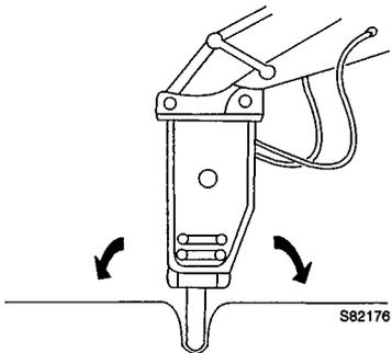
Do not bend with the chisel to make a hole in the ground.
