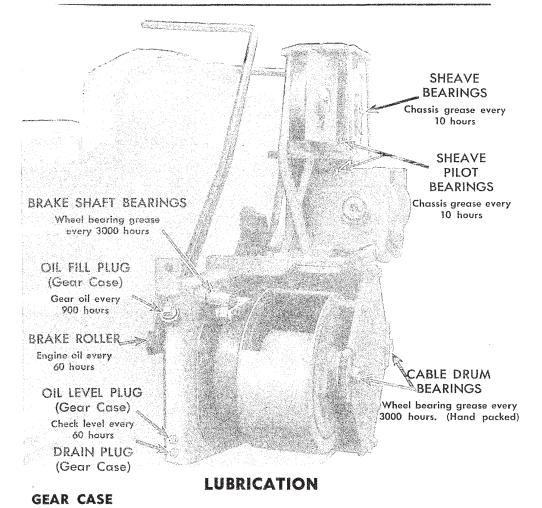
All gears, bearings, and working parts inside the Power Control Unit gear case receive lubrication by the "splash" system from the oil in the lower part of the case. The main gears dip in the oil when turning and the constant spray of oil resulting therefrom provides ample lubrication.
