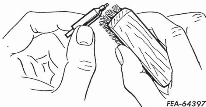
Illust. 64. Cleaning and polishing valve and pintle.
