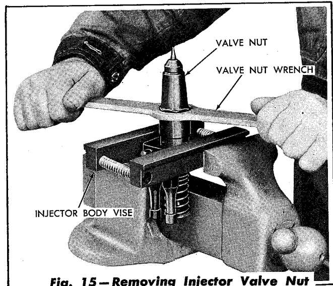
Fig. 15 — Removing Injector Valve Nut
