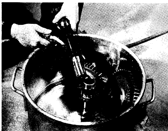
53 Clean carefully with clean solvent. Blow off parts with dry compressed air.
