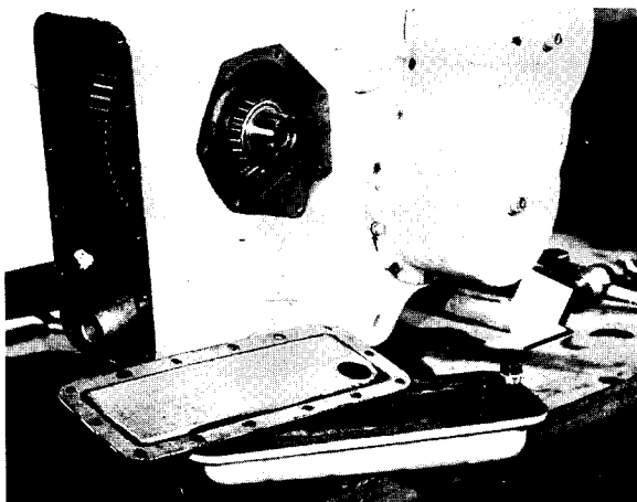
43 Sump cover and oil screen, removed. Clean screen, sump and magnetic plug.
