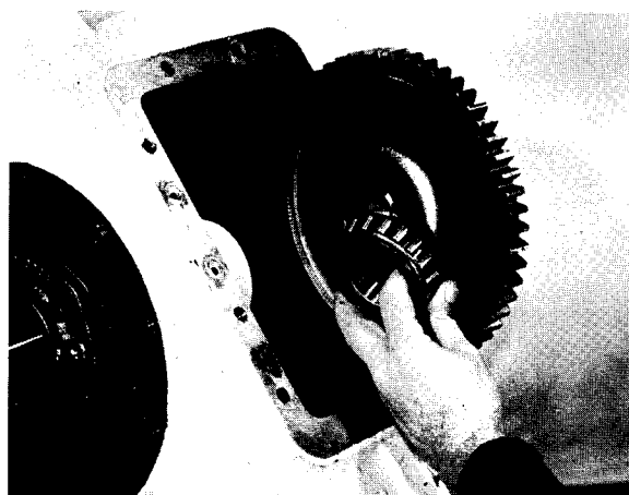
38 Remove high speed gear and bearing.
