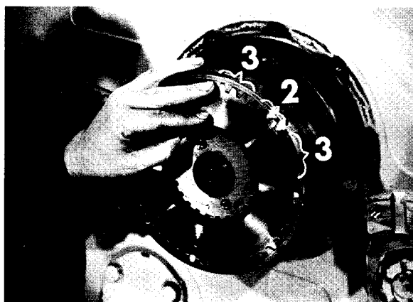
27 The first disc is always a steel one. The teeth are in groups of three, except for one spot. At this one spot, either two or four teeth will be found, depending on the model tractor shovel. Clutch illustrated has only two. As discs are installed, mark drum as illustrated. As you put in the disc, put down two chalk marks as shown.
