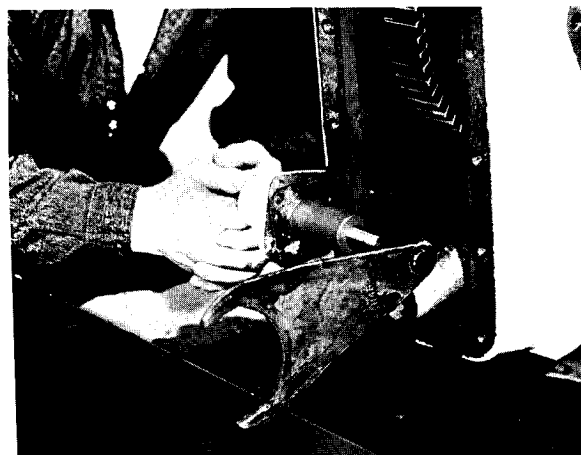
44 Remove shift shaft and fork.
