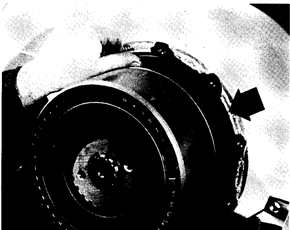
33 Install new "O" ring.
