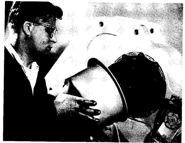
14 Remove clutch housing.
