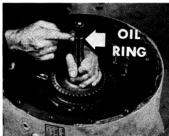
40 Install new steel oil ring. Insert shaft with ring up. Press bearing race in position with tapered side out.
