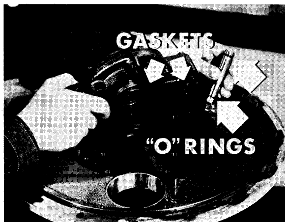
41 If oil pump is questionable, install new pump. Always replace "O" rings and gaskets.
