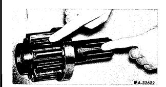
Inspect for wear, chips, cracks, or burrs. Worn pinions may be used on the other side of the tractor if they are not chipped or cracked.
