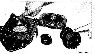
Inspect for scores, cracks, wear, or looseness. Replace if not fit for further use. Lubricate bearing surfaces and wrap until ready for assembly.
