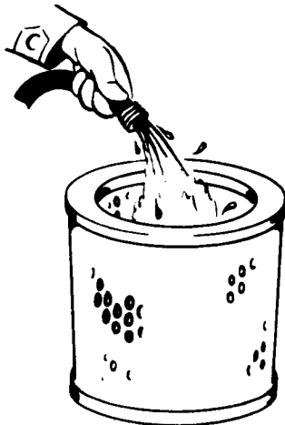
Removing dust with water hose.
