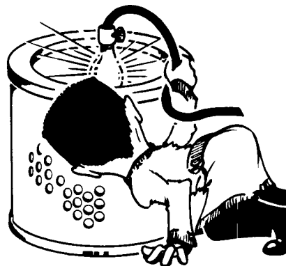
Inspecting element with bright light.
