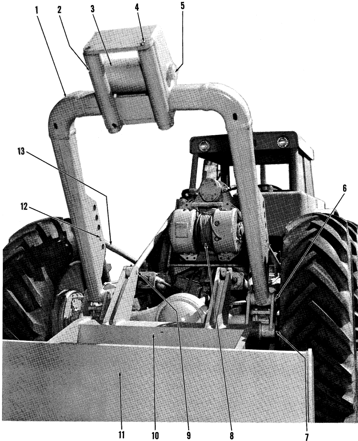
"A" FRAME, DOZER BLADE AND UPPER ARM
