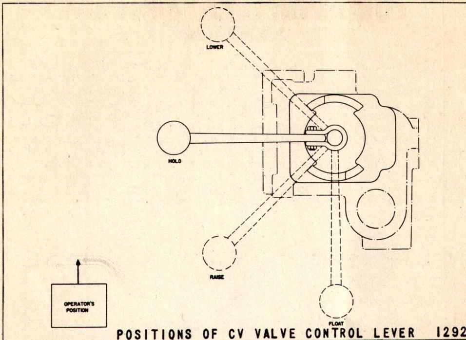
4. "Float" position - lever may be moved back or forward 90° from "Hold" position, or parallel with the line of travel of the tractor. (Note: the valve has two "Hold", two "Hoist", two "Down" and two "Float" positions, since the control lever can be reversed to the opposite side of the valve. Either position may be used with the same accuracy of control.
