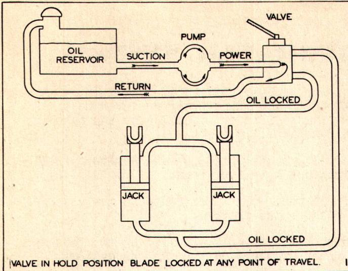
1. Valve Hold Position. We find by consulting this simple diagram that the oil (follow the arrows in the line) leaves the tank and flows by gravity and suction through the low pressure hose called "suction line" to the intake port on the pump where it is picked up by the teeth of the gears
