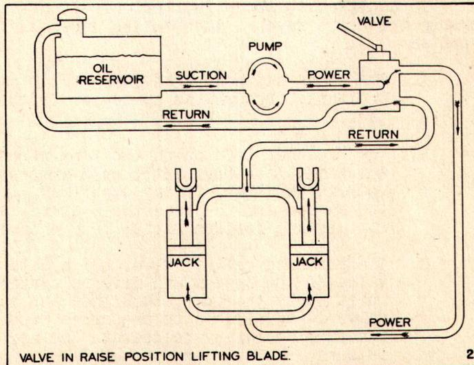
2. Valve - Raise Position. By following the course of the arrows we find in this illustration that oil from the power line is being diverted by the control valve from entering the tank, and is proceeding instead, to the base or bottom end of the jack cylinder while oil from the top end of the jack cylinder is being forced, by the advancing piston, through the line to the control valve and back into the tank.
