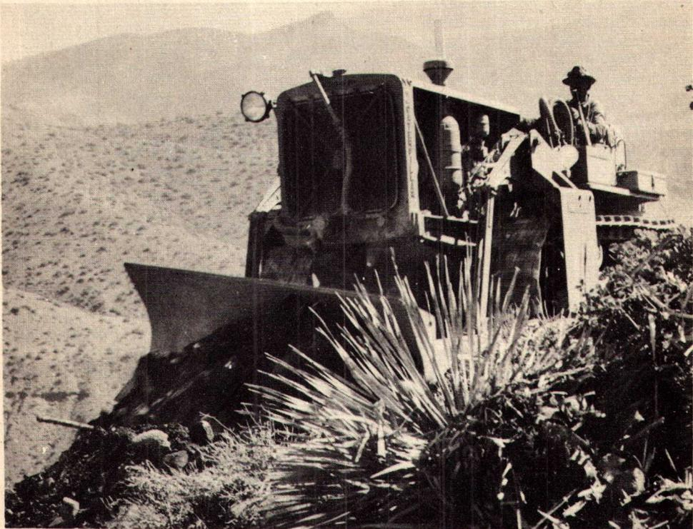
Trailbuilders are primarily designed for pioneering trails through hilly or mountainous country, for clearing right-of-way for roads, airports, camp-sites, reservoirs, training bases and similar projects. They are especially useful in the construction of ramps and in the building of trails through dense jungle. Handling rocks, logs, stumps and debris is easy and practical with these efficient units.
