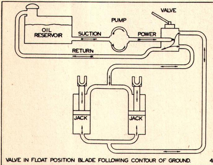
4. Valve Float Position - In this position the ports of the control valve are open allowing oil to flow freely from one end of the jacks to the other end, cross between the two jacks, or enter the return line to the tank, thus enabling the blade to raise or lower freely accord-
