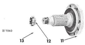
SHAFT less oil seal guard, bull gear (2) (for use on machines prior to serial No. 3673 when equipped with Oil Seal, 635 084 R91)(for service supply 1-636 804 R91, Bull Gear Shaft Service Package; 1-636 496 R91, Oil Seal Service Package and 1-636 491 R1 Spacer Ring)
