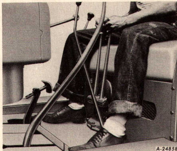
Illust. 30 Both hydraulic control levers pulled all the way back to "lock" both tracks.
