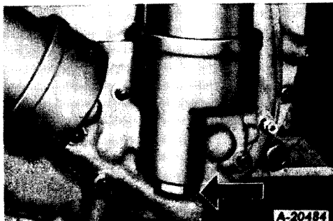
Item 13 - Transmission and planet power drive filter drain plug.
