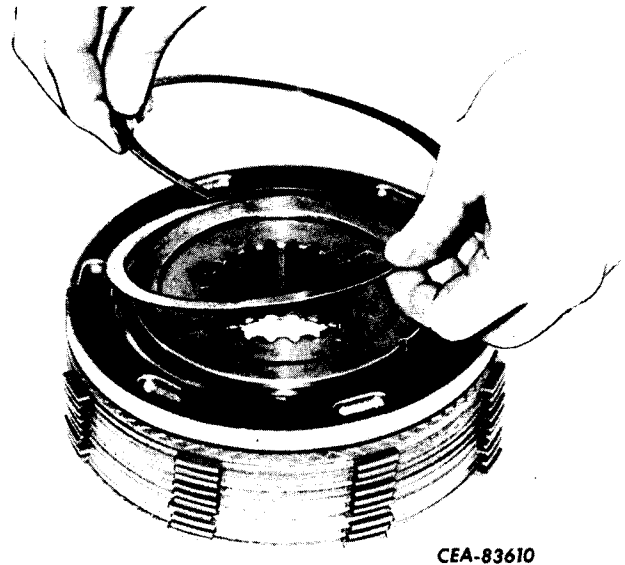
Illust. 43 Removing the Clutch Hub Spiral Snap Ring.
