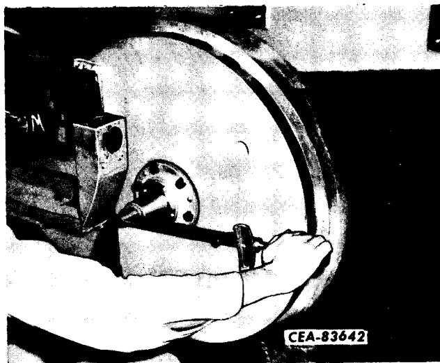
Illust. 30 Checking Front Idler Bearing Pre-load.
