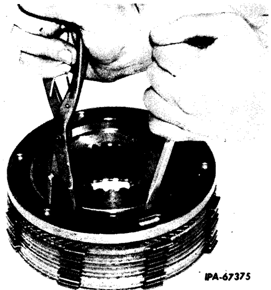
Illust. 44 Removing Clutch Hub External Snap Ring.
