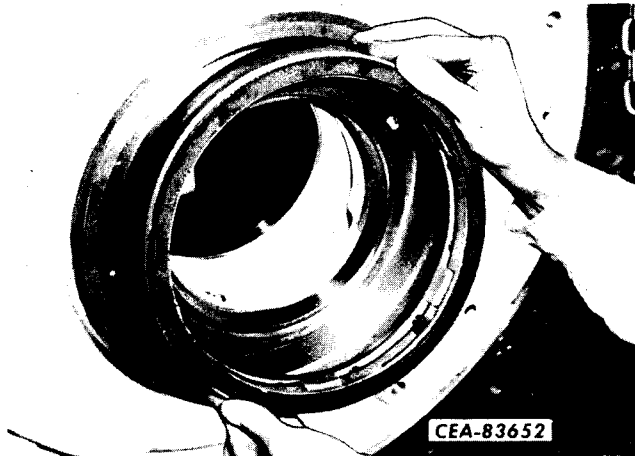
Illust. 9 Removing the Seal Rotor from the Sprocket Carrier (Spring Loaded Rubber Face-Type Oil Seal).
