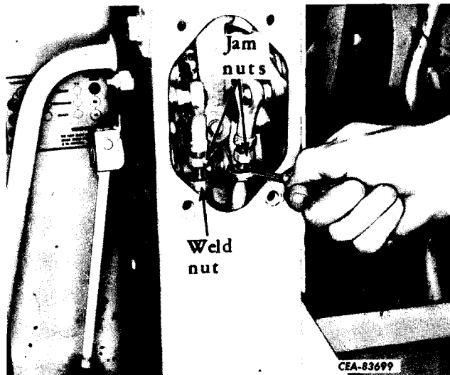
Illust. 76 Turning Upper Adjusting Links to Connect at Lower Bell Cranks.
