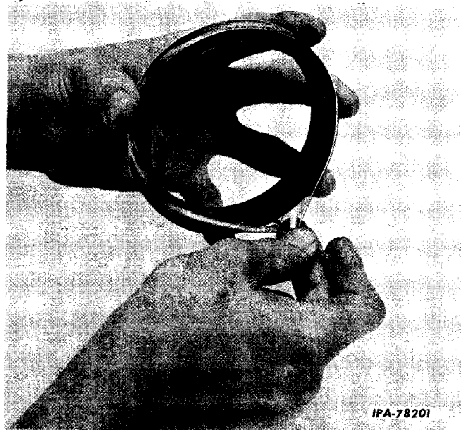
Illust. 27 Installing Unitization Band on Metal Rings.
