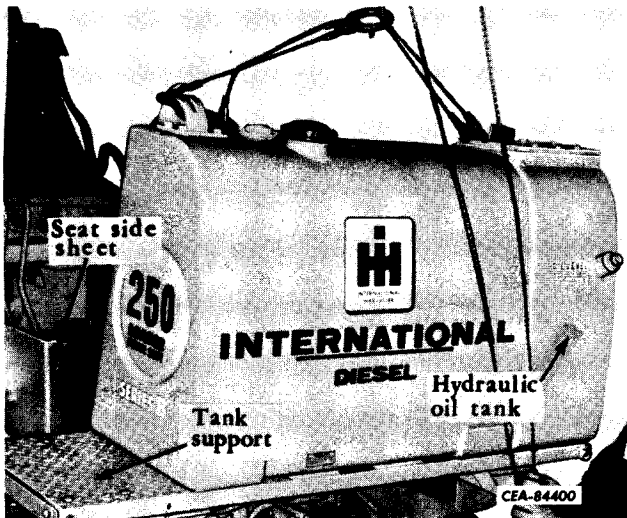
Illust. 4 Removing the Fuel Tank and Hydraulic Oil Tank as an Assembly.
