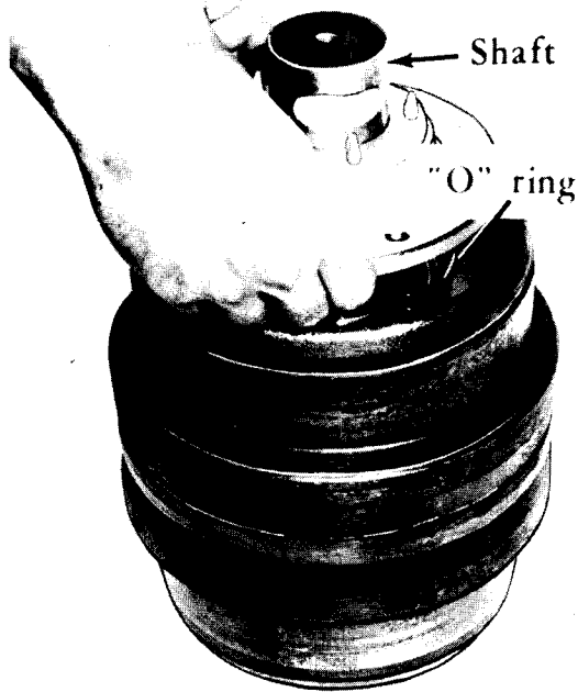
Illust. 47 Removing the Track Idler Oil Seal.
