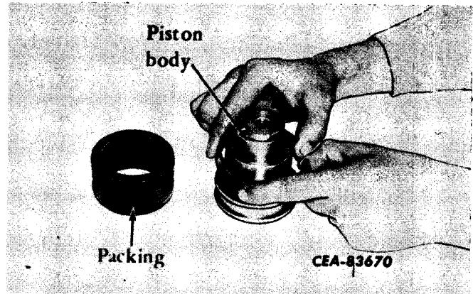
Illust. 38 Removing the Piston Body Wear Ring.
