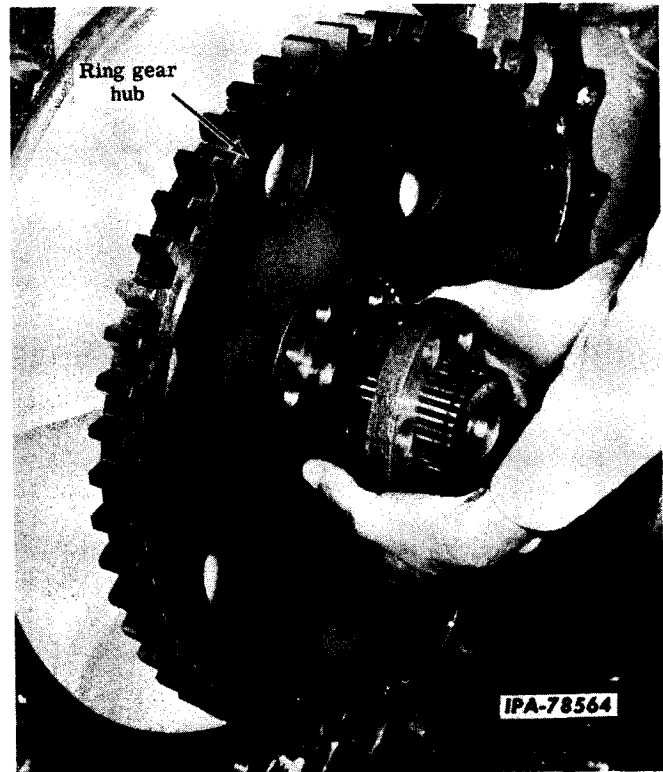
Illust. 5 Removing the Bearing Retainer Plate and Shims.
