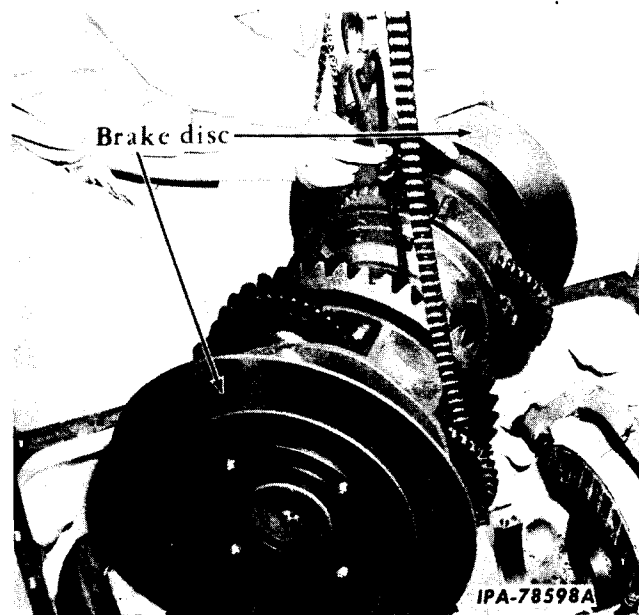
Illust. 9 Removing the Steering Planetary from the Rear Main Frame.
