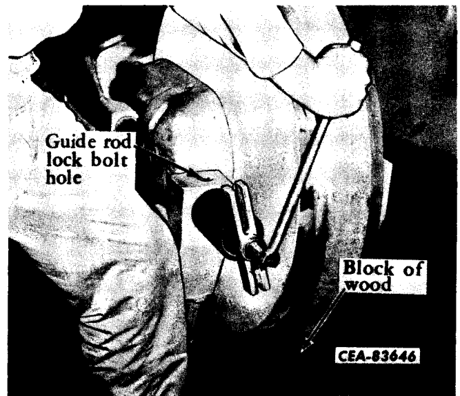
Illust. 15 Removing the Front Idler Guide Rod.
