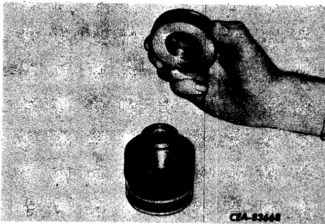
Illust. 36 Removing the Piston End.
