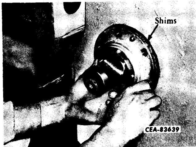
Illust. 29 Installing the Front Idler Oil Seal.
