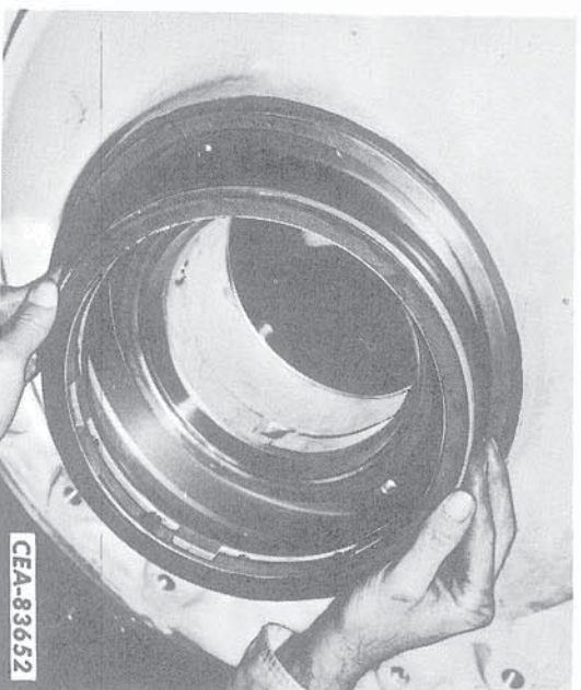
Illust. 9 Removing the Seal Rotor From the Sprocket Carrier.
