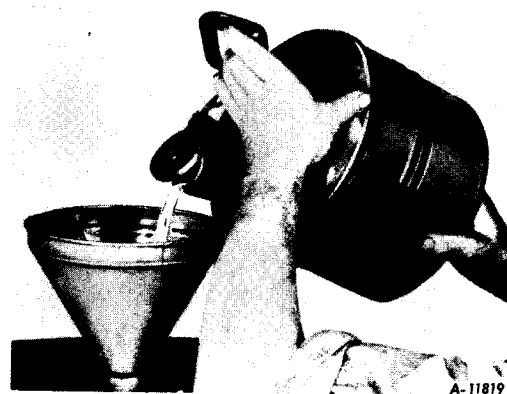
Illustr. 14 Correct method of pouring gasoline into the tank.
