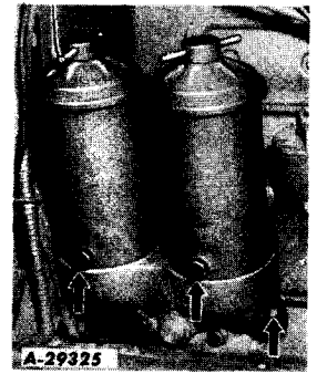
Item 34 - Lubricating oil filter drain plugs. Drain the filter base and filter cases whenever the crankcase oil is drained. Drain the oil while the engine is hot. After replacing the plugs, add 1 quart of oil to each case. The 2 quarts added should be deducted from the total amount required for the crankcase.
