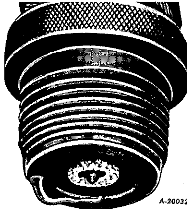
Illustr. 6 - Badly Burned (Pre-ignition or Poor Cooling).
