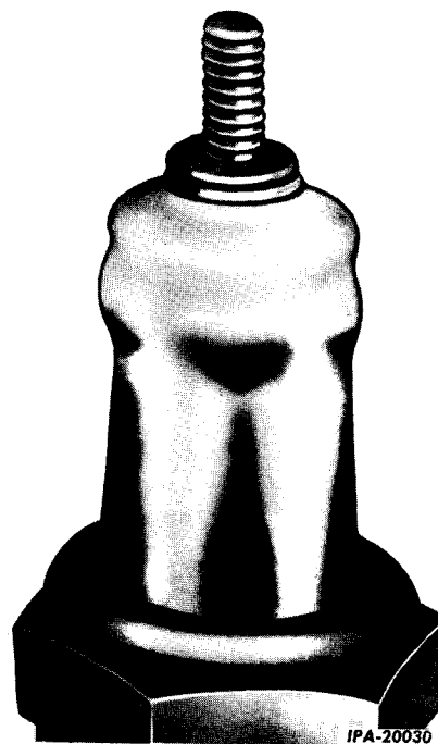
Illust. 4 - Streaked Insulator Top (Blow-by).
