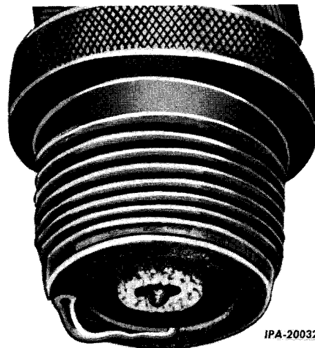
Illust. 5 - Badly Burned (Pre-ignition or Poor Cooling).
