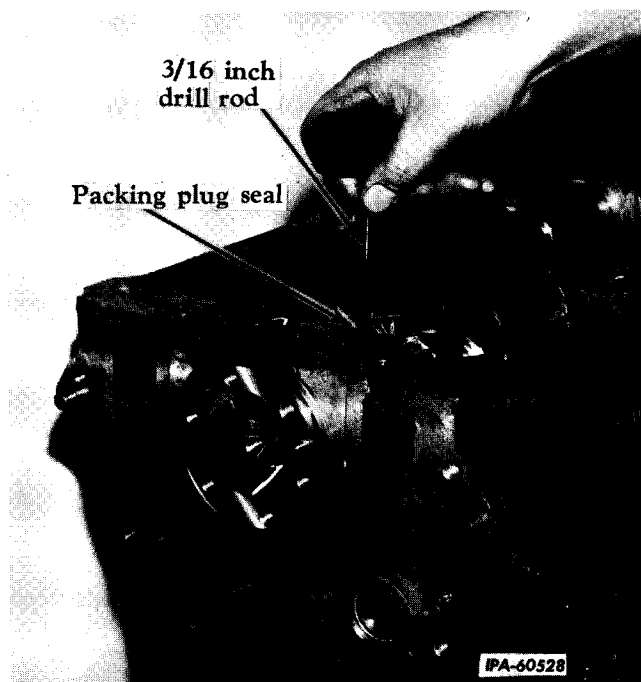
Illustr. 12 - Installing the Rear Main Bearing Cap Packing Plugs.
