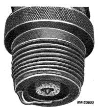
Illust. 6 - Badly Burned (Pre-ignition or Poor Cooling).
