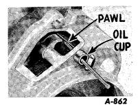
Illust. 36 - View Showing How the Main Pawl Can Be Lifted, Disengaging The Impulse Coupling for Free Rotation During Timing.
