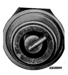
Illust. 3 - Carbon Coating (Rich Mixture, Oil Pumping, or Cold Plug).
