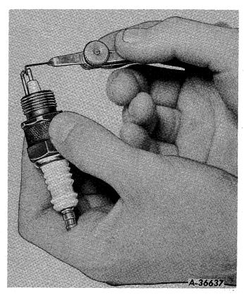
Illust. 1 - Checking Diesel Engine Spark Plug Gap.
