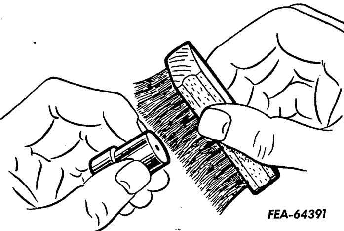
Illust. 57. Cleaning and polishing valve body (orifice end).
