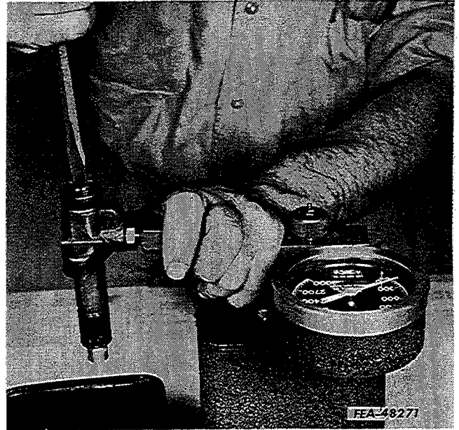
Illust. 67. Adjusting nozzle opening pressure.
