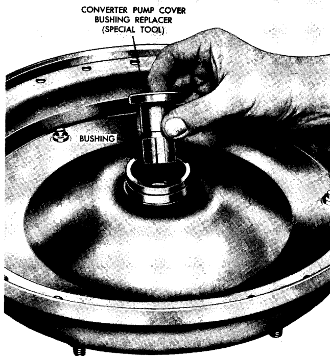
Fig. IX-5 Installing pump cover bushing
