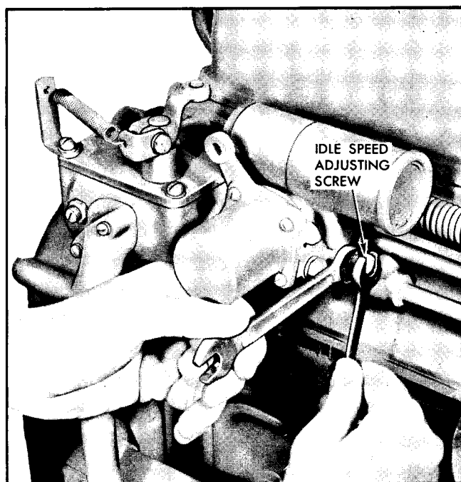
Fig. 4 - Adjusting Idle Speed
