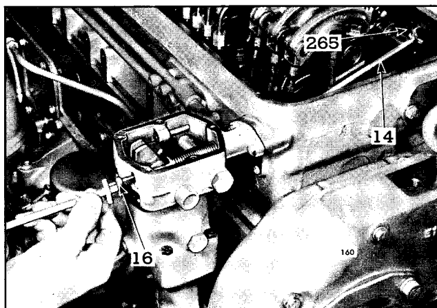
Fig. 1 - Adjusting Fuel Rod
