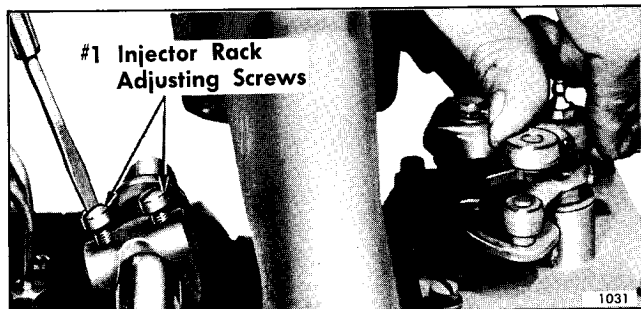
Fig. 8 - Adjusting No. 1 Rack to Governor
