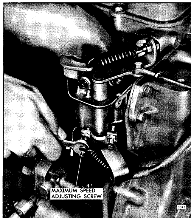
Fig. 6 - Adjusting Maximum No-Load Engine Speed
