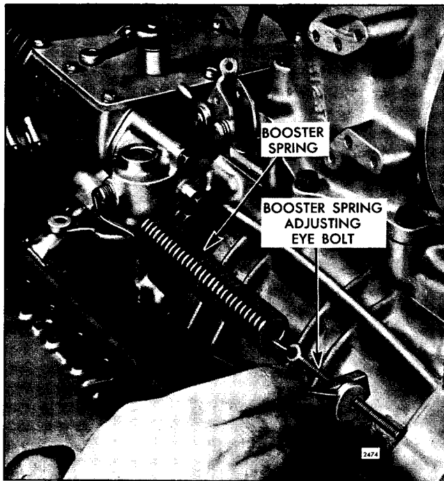
Fig. 5 - Adjusting Booster Spring
