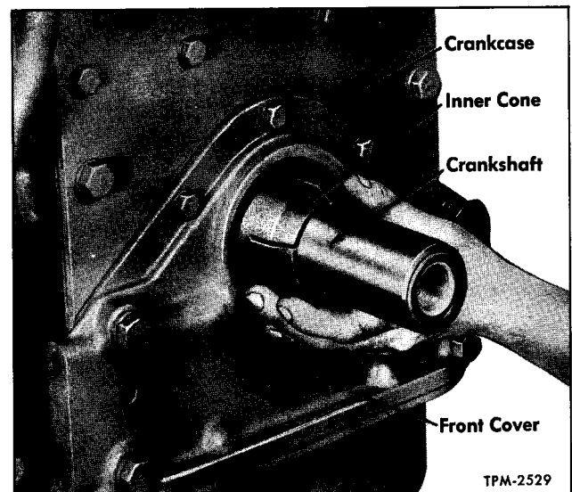
Figure 33—Installing Oil Seal Spacer (Inner Cone)
