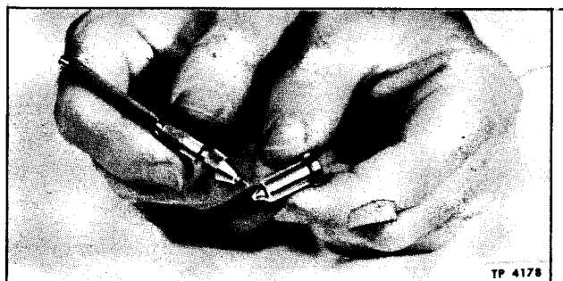
Figure 23—Cleaning Spray Tip Orifices
