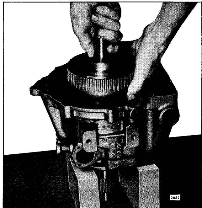
Fig. 24 - Removing Drive Gear Input Shaft, Forward Clutch and Ring Gear Assembly from Reverse Gear Housing
