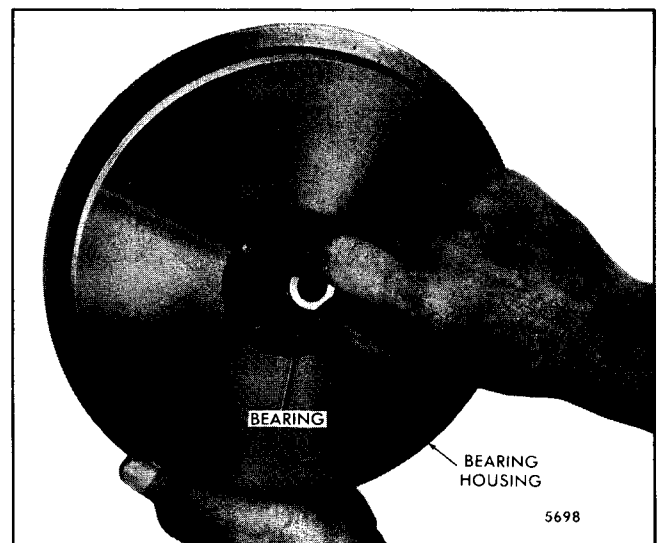
Fig. 10 - Removing Turbine Shaft Bearing from Bearing Housing
