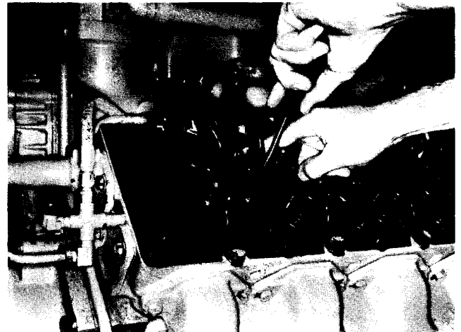
Fig. 2-33, (V11915). Adjusting crossheads
