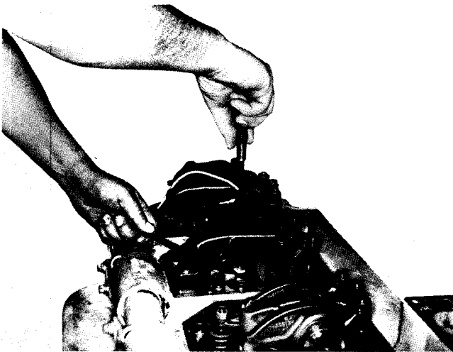
Fig. 2-55, (K114105). Adjusting crosshead to slave piston clearance
