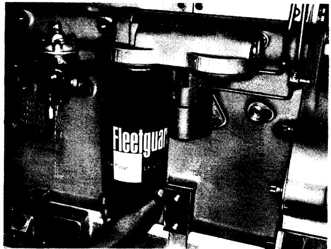
Fig. 2-15, (K11951). Removing "spin-on" lubricating oil filter — KT(A)-1150 Engine
