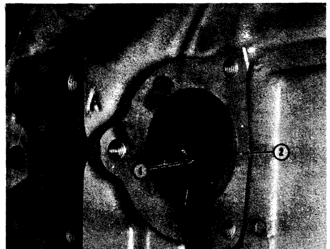
Fig. 2-60, (K21918). Valve set marks on right bank flywheel and housing — KT(A)-2300
