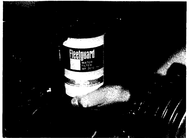
Fig. 2-23, (V514132). Installing DCA "spin-on" water filter
