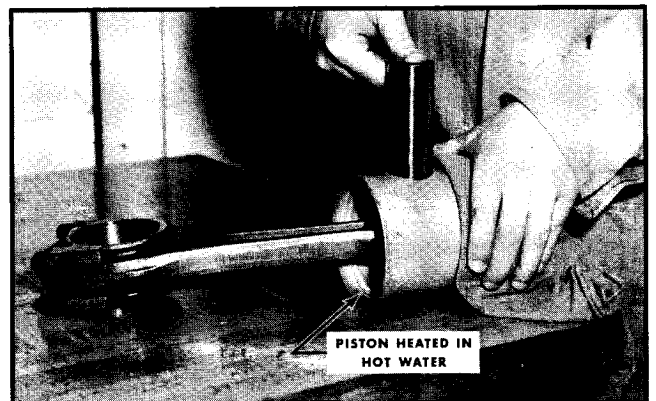
Fig. 12-18. Installing piston pin
