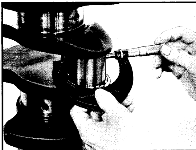
Fig. 2-18. Measuring crankshaft journal
