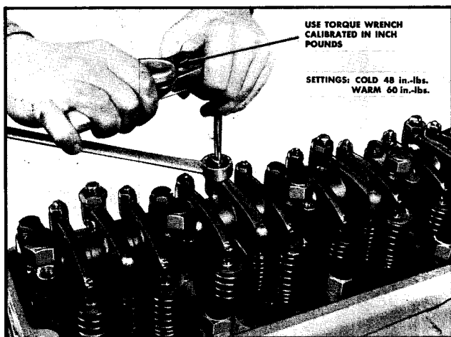
Fig. 12-64. Adjusting injector plunger
