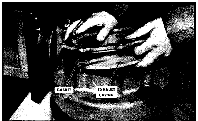
Fig. 10-13. Removing turbo exhaust casing and gasket
