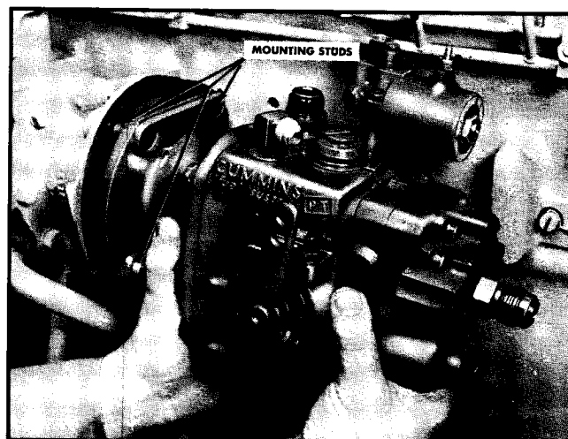
Fig. 12-81. Mounting fuel pump
