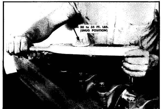
Fig. 12-7. Snug tighten to 30-35 ft. lbs.
