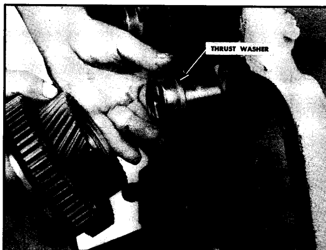
Fig. 12-28. Installing thrust washer and idler gear assembly
