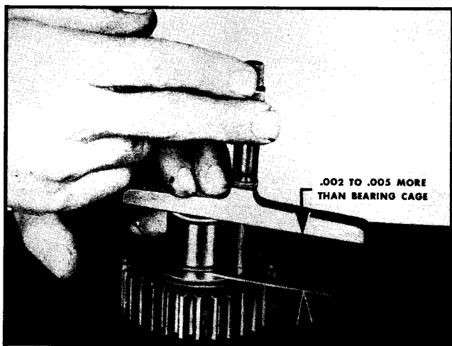
Fig. 10-8. Checking hub length for end play
