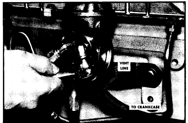
Fig. 12-99. Installing vent line to crankcase
