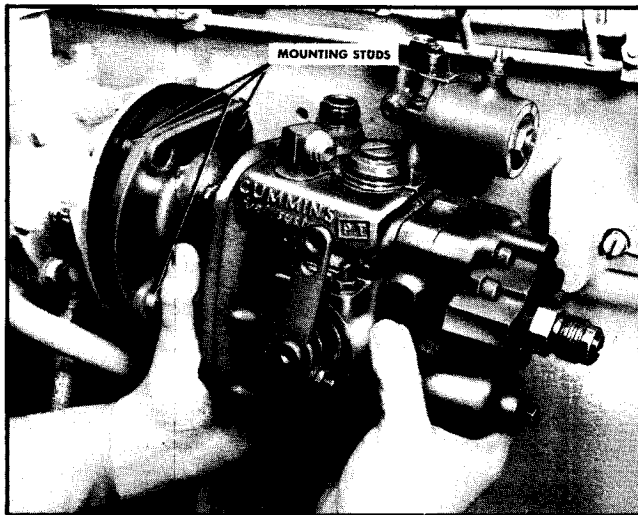
Fig. 1-6. Remove fuel pump
