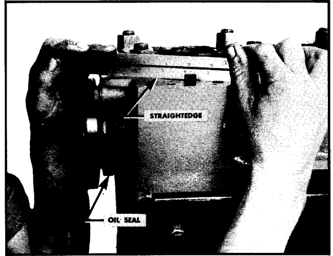
Fig. 12-11. Checking rear cover plate alignment
