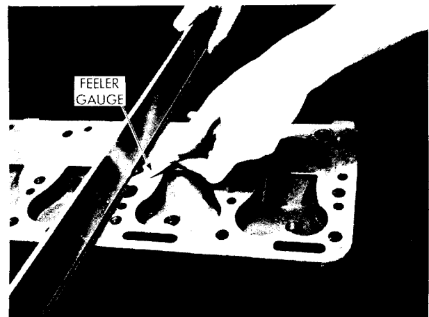
Figure 112 — Checking cylinder head flatness crosswise.
