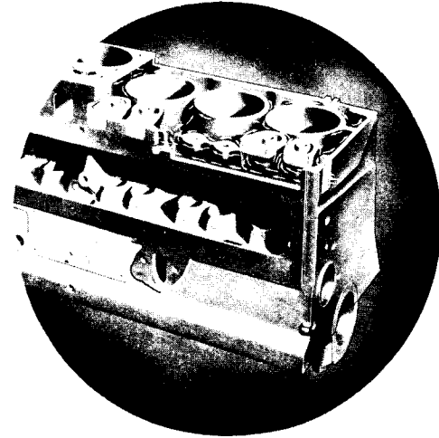
Figure 12 — Directional Cooling in Block
