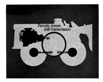
They permit the use of a power shift transmission which can permit quick gear changing even under load.
