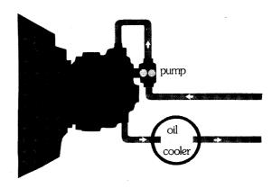
The oil cooler receives hot oil from the converter, cools it and returns it to the system. Coolers also create some back pressure which helps to keep the converter full of oil. To understand how back pressure helps to keep the converter full, consider this example.
