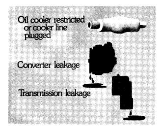
a converter oil cooler plugged, a restriction in the cooler lines, excessive converter leakage and excessive transmission leakage.
