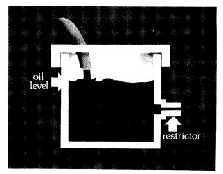
Some converters are also fitted with a down stream regulator valve. The oil leaving the converter must push the down stream regulator spool against a spring. This creates back pressure within the converter and keeps it full of oil.
