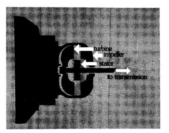
Suppose that your machine is traveling on a smooth flat surface with no load and the engine is turning at 2000 RPM. The impeller, because it is connected directly to the engine, is also turning at 2000 RPM and with no load, the turbine matches that 2000 RPM speed. With the turbine and impeller rotating at the same speed, each create the same centrifugal force.
