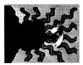
Like all other man-made machinery, the Torque Converter is not 100 per cent efficient. Because the members are not mechanically connected, there is some oil slippage and the result is heat.
