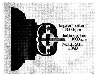
But even after the oil flows through the turbine, it is still moving rapidly and has force. This is where the stator comes in.
