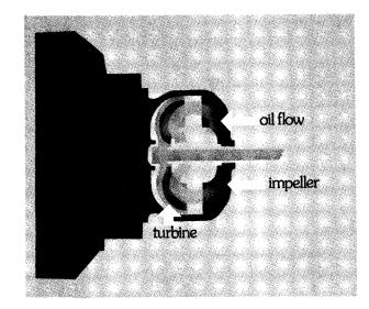
This outward flowing oil leaves the impeller and strikes the blades of the second fan called a turbine, so you can see that it is the force of this flowing oil that causes the turbine to rotate. This fluid coupling is complete and energy is transmitted from one member to the other through oil flow.
