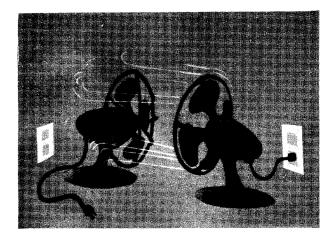
Hydrodynamic systems work on the principle that a fluid in motion has force. For instance if you look at two fans facing each other and one is plugged in and the other isn't, you would see that the electrically driven blades were forcing air toward the blades of the unplugged fan. This flow of air has force which makes the blades of the unplugged fan rotate.
