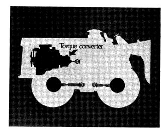
A Torque Converter is a device which transmits force and motion from an engine to a transmission by means of hydraulic oil. There are really only two kinds of systems that transmit energy hydraulically.
