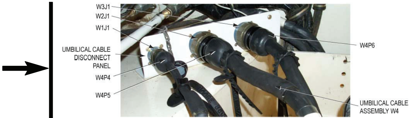
Figure 25. Umbilical Cable Assembly W4 Connection to Umbilical Cable Disconnect Bracket
