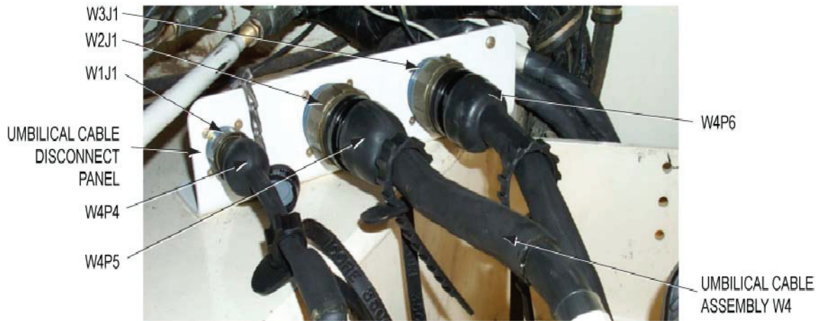
Figure 30. Umbilical Cable Assembly W4 Connection to Umbilical Cable Disconnect Bracket
