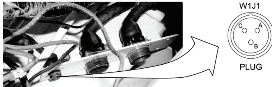
Figure 15. Location of Power Cable Assembly Connector W1J1
