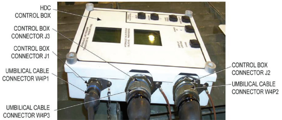
Figure 2. Umbilical Cable Assembly W4 Connections to HDC Control Box
