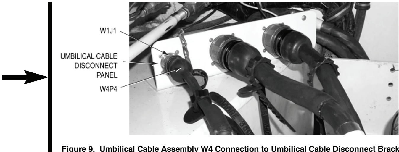
Figure 9. Umbilical Cable Assembly W4 Connection to Umbilical Cable Disconnect Bracket
