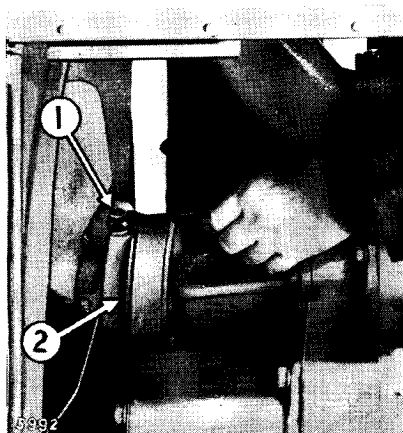
FAN BELT ADJUSTMENT 1—Lock screw. 2—Adjusting rim.
