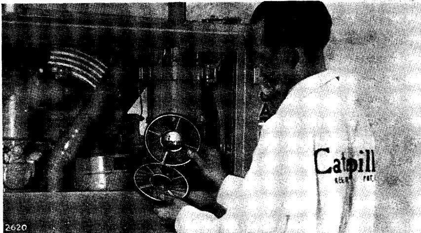
ALIGNING AIR CLEANER SCREENS
