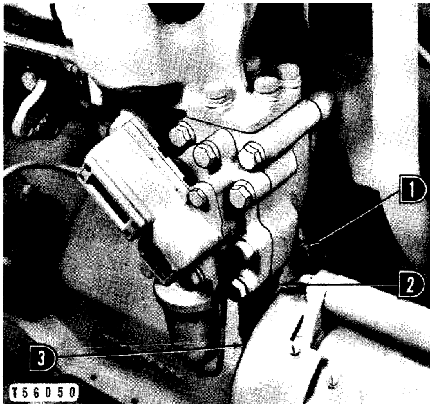
PREPARING TO REMOVE THE FUEL TRANSFER PUMP
