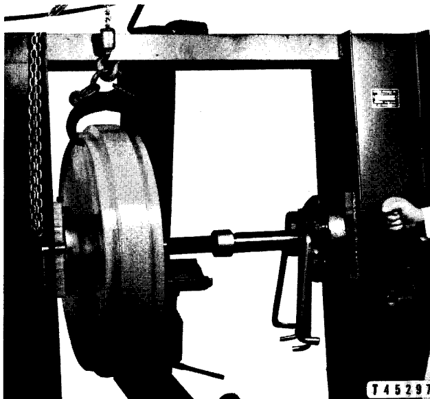
PREPARING TO REMOVE FRONT IDLER BUSHING
