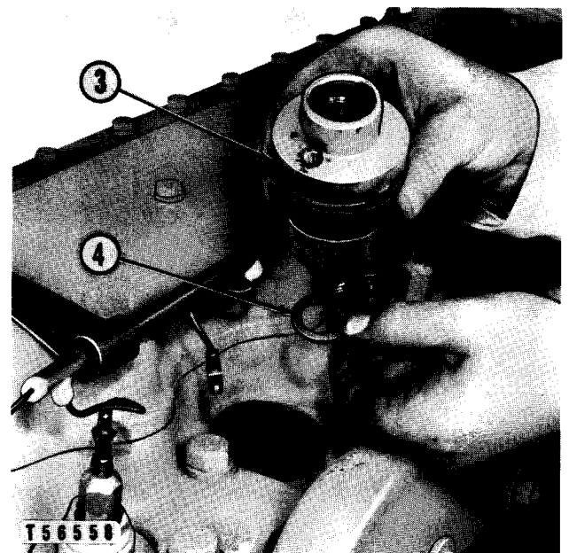
REMOVING PRECOMBUSTION CHAMBER EQUIPPED WITH GLOW PLUG 3-Precombustion chamber. 4-Gasket.
