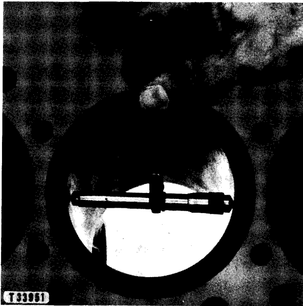
CHECKING LINER WEAR
