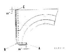
b) Put the seal in the groove of the cap at point (A). Work the seal around point (B) to point (C). Do not pull on the seal. Make sure the seal
