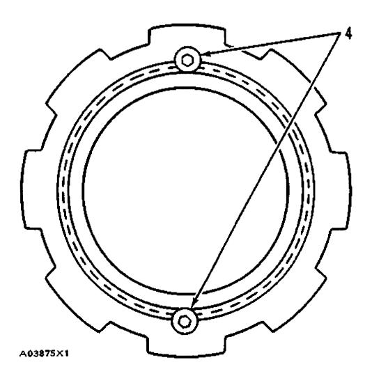
4. Use a 1/4"-20-3B NC thread tap to tap both holes .31 in. (7.9 mm) deep. Instal two screws (4).
