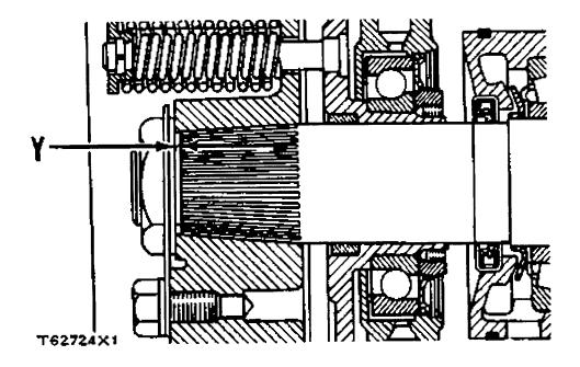
12. Remove tooling (C). Measure dimension (Y). Dimension (Y) must be .22  $\pm$  .03 in. (5.6  $\pm$  0.8 mm).
