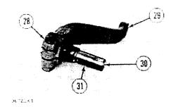
**20.** Remove bolt and nut (28) from right hand lever (29). Remove shaft (30) and key (31).
