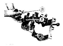
14. Install two bearing races (21) and bearing rollers (20).
