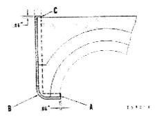
**b)** Put the seal in the groove of the cap at point (A). Work the seal around point (B) to point (C). Do not pull on the seal. Make sure the seal
