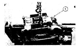
**1.** Fasten a hoist to the steering clutch controls. Put the steering clutch controls (1) in position on the steering clutch case.
