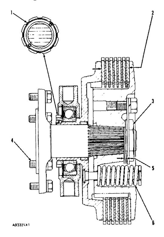
(1) Torque for the nut that holds the bearing in the cage . . . 350  $\pm$  50 lb.ft.
