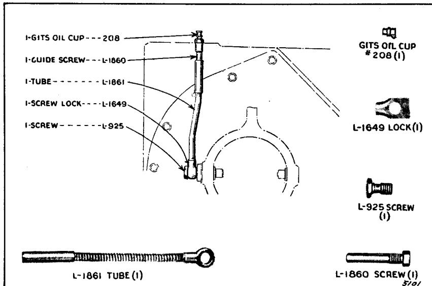
STEERING CLUTCH RELEASE BEARING OIL TUBE (2 Groups Req'd.)
