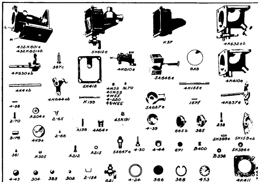
"CATERPILLAR" No. 2A1701 CARBURETOR (Gasoline or Tractor Fuel)
