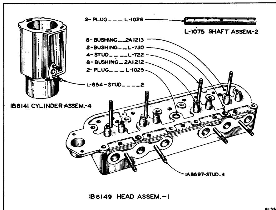
CYLINDER, CYLINDER HEAD AND VALVE MECHANISM ASSEMBLIES
