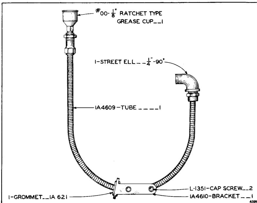
FLYWHEEL CLUTCH RELEASE BEARING OIL TUBE
