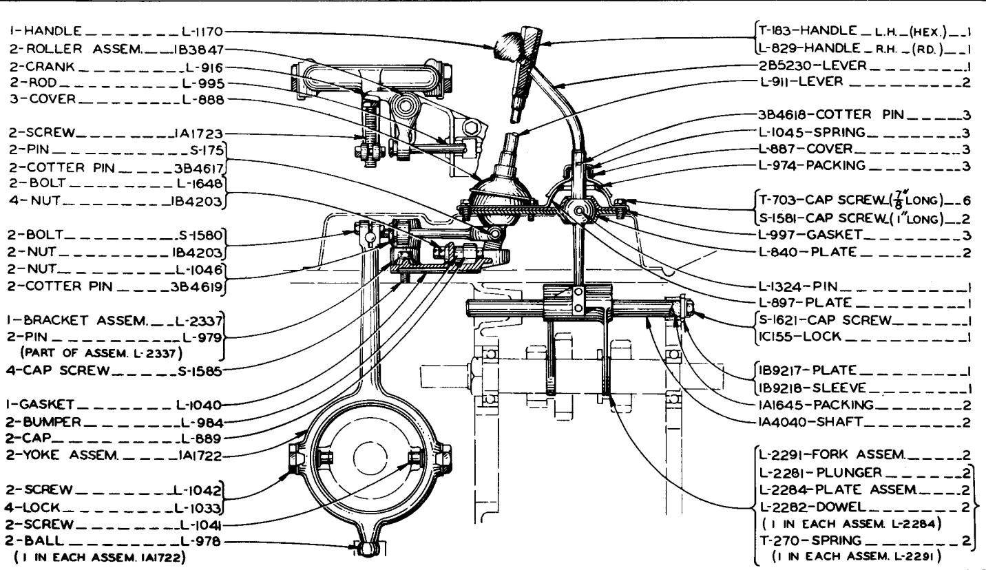
GEAR SHIFT AND STEERING CLUTCH CONTROL
