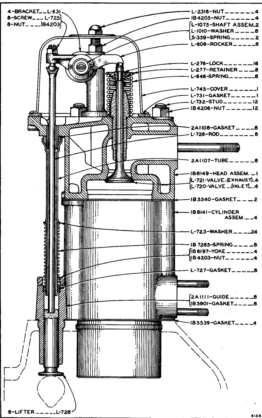
CYLINDER, CYLINDER HEAD AND VALVE MECHANISM
