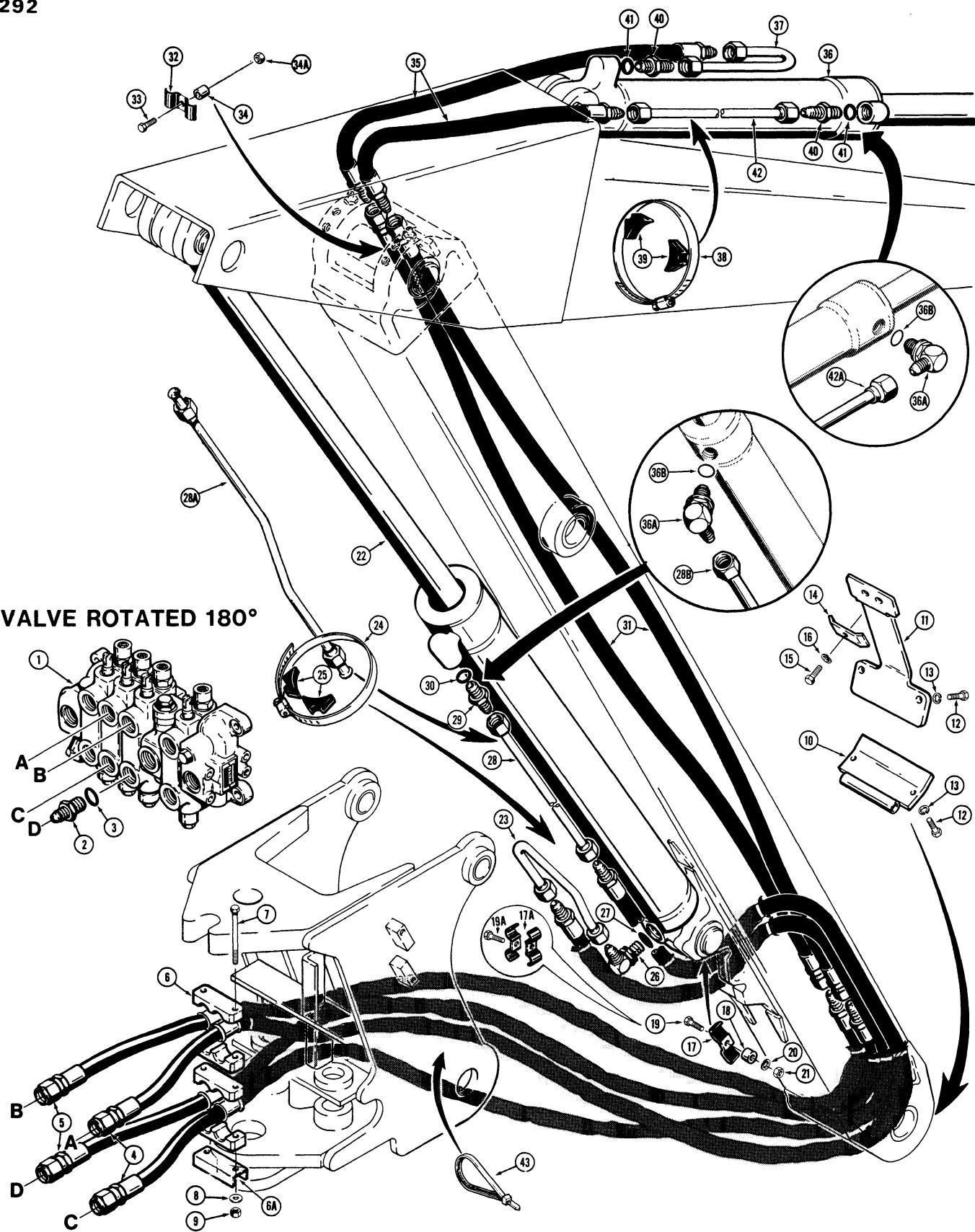
**BACKHOE DIPPER AND BUCKET CYLINDER HYDRAULIC CIRCUIT**
