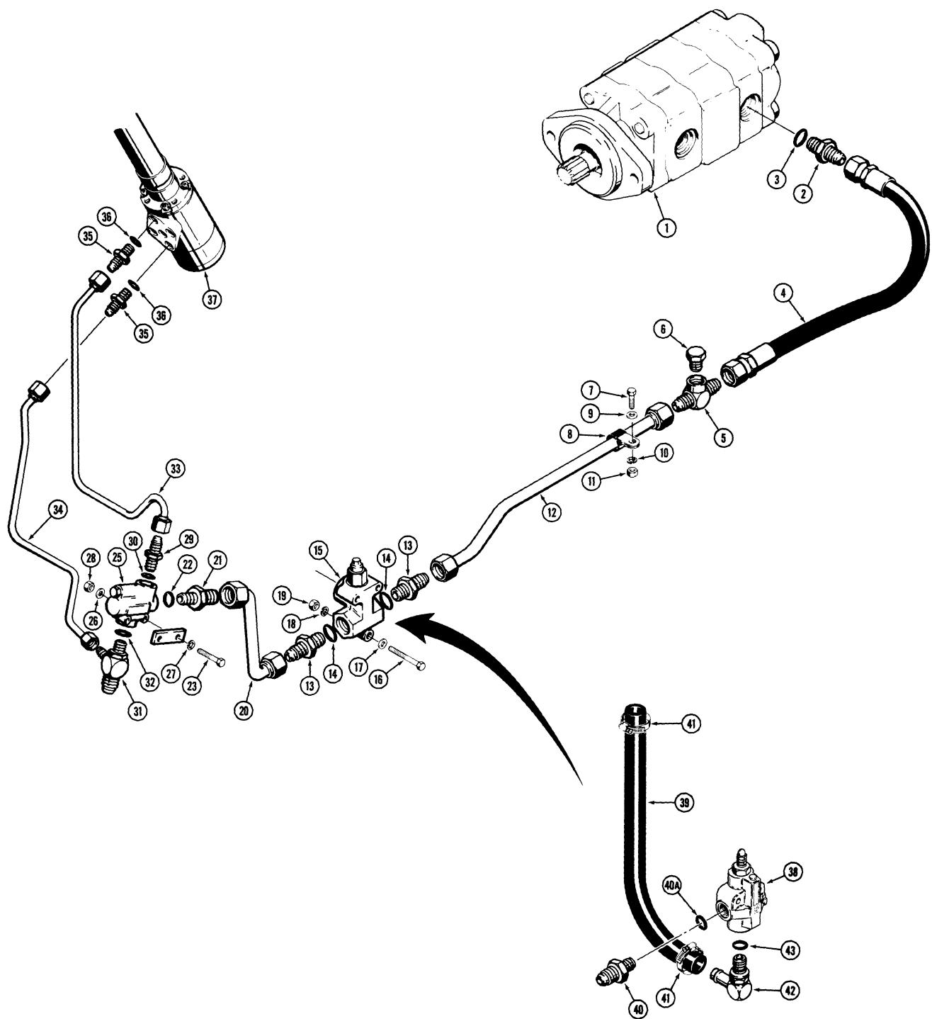
**STEERING VALVE HYDRAULIC CIRCUIT**
