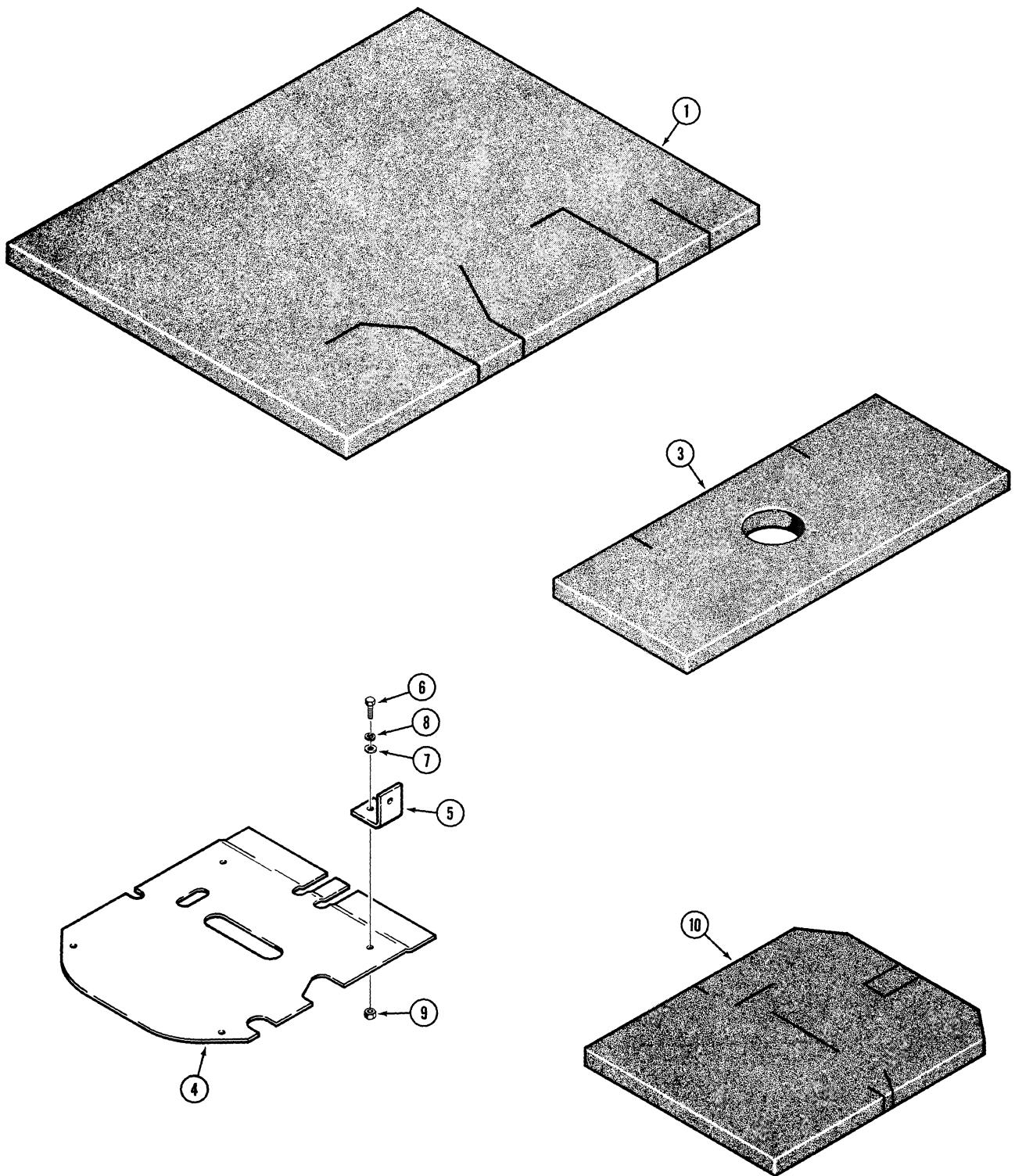
**MODEL 680E CONSTRUCTION KING LOADER BACKHOE 457****NOISE REDUCTION PADS**
