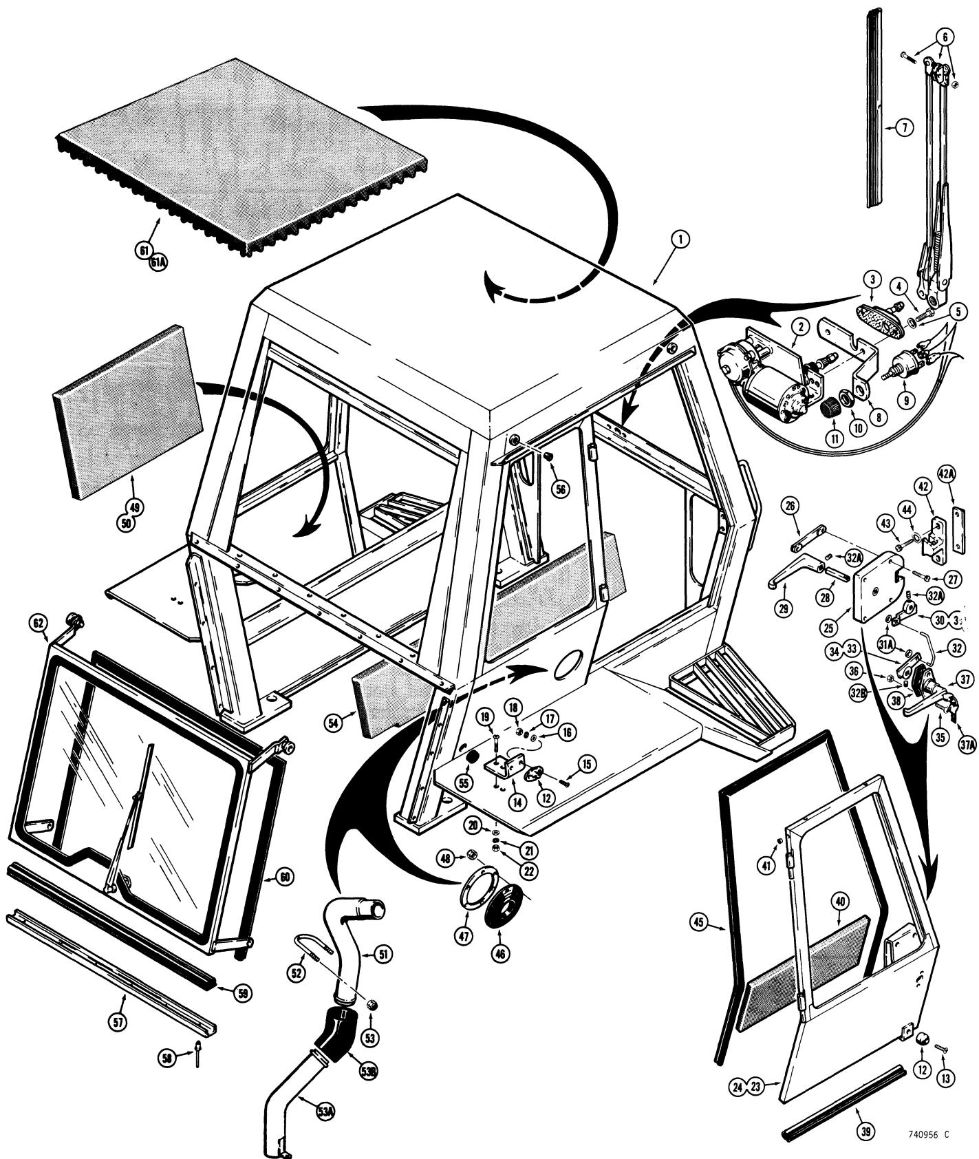
**\*OPERATOR'S CAB (CASE BUILT)
