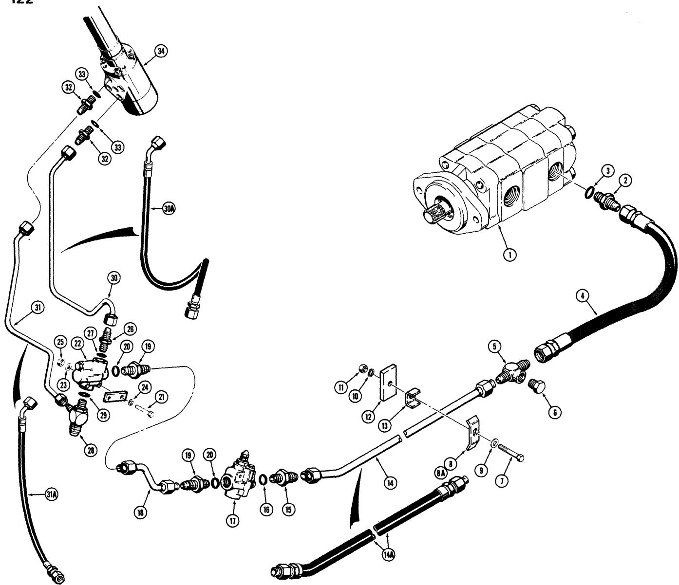
**STEERING VALVE HYDRAULIC CIRCUIT**
