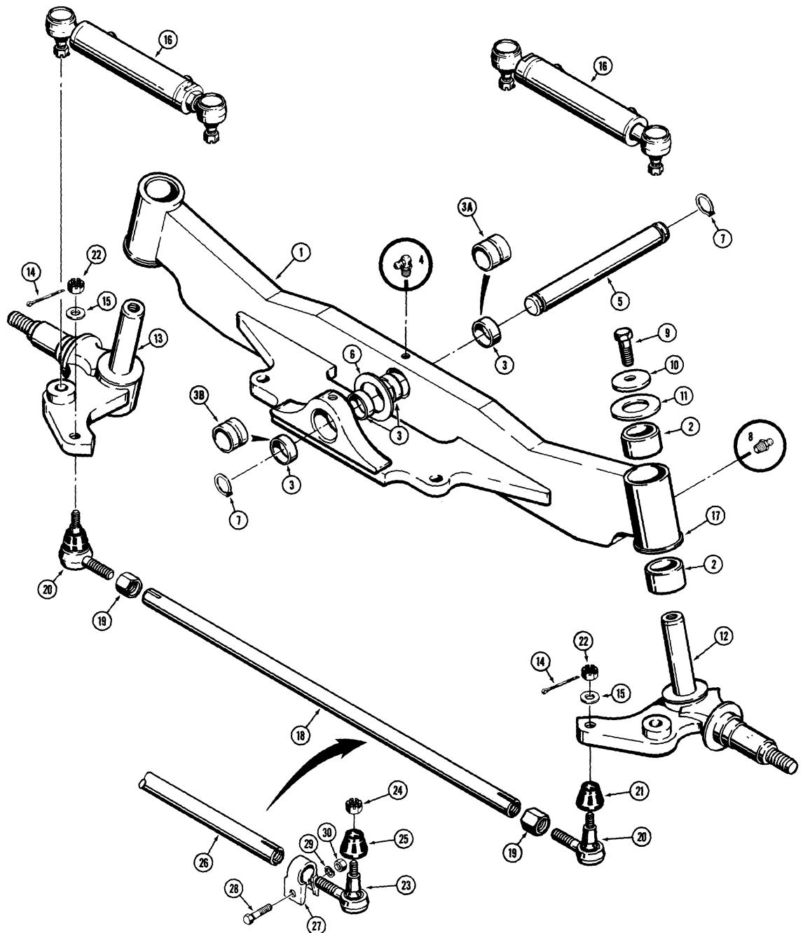
**FRONT AXLE, SPINDLES AND TIE ROD****MODELS WITH CLAMP RETAINED BALL JOINTS TO TUBE**
