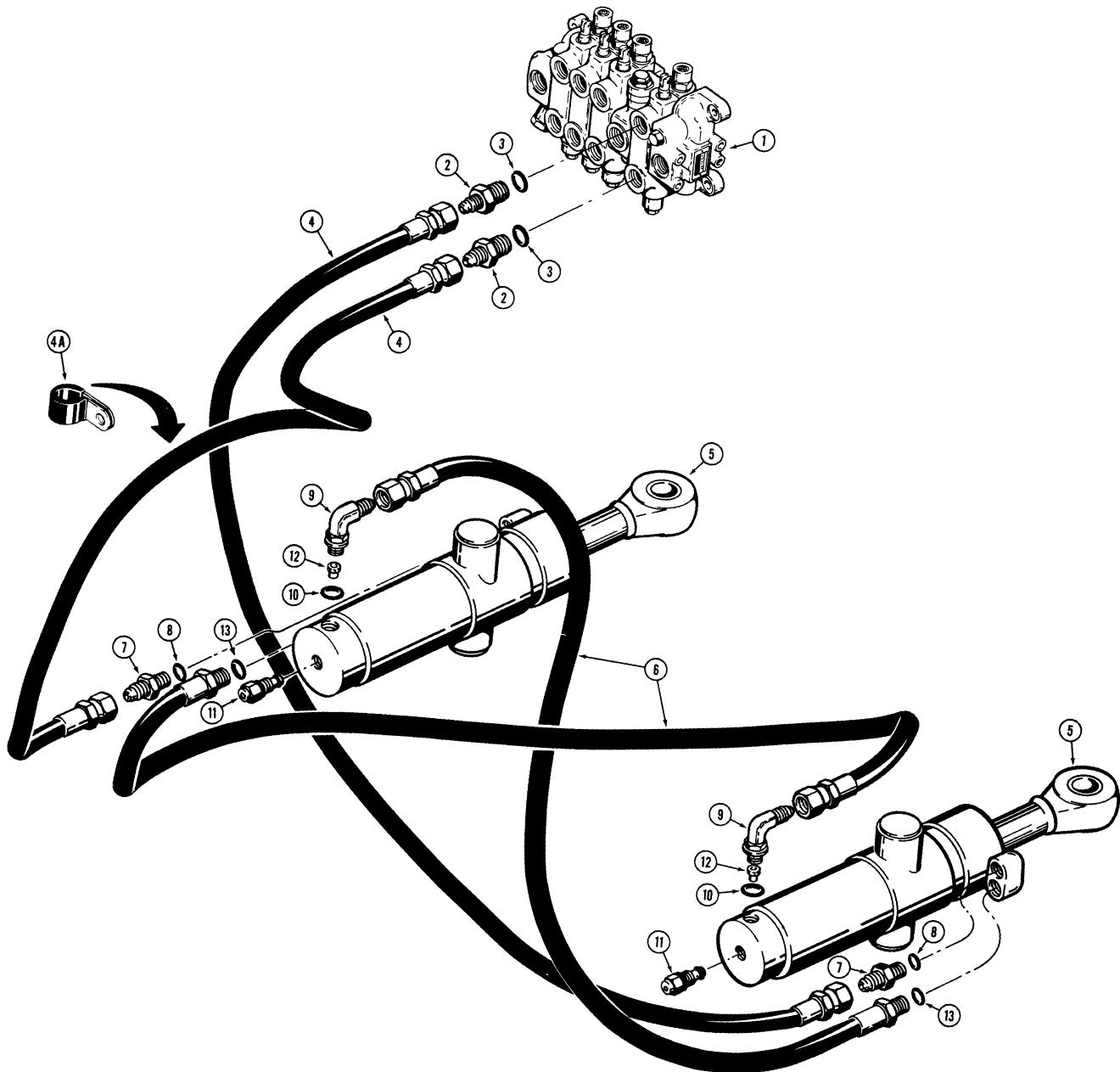
**BACKHOE SWING CYLINDER HYDRAULIC CIRCUIT**
