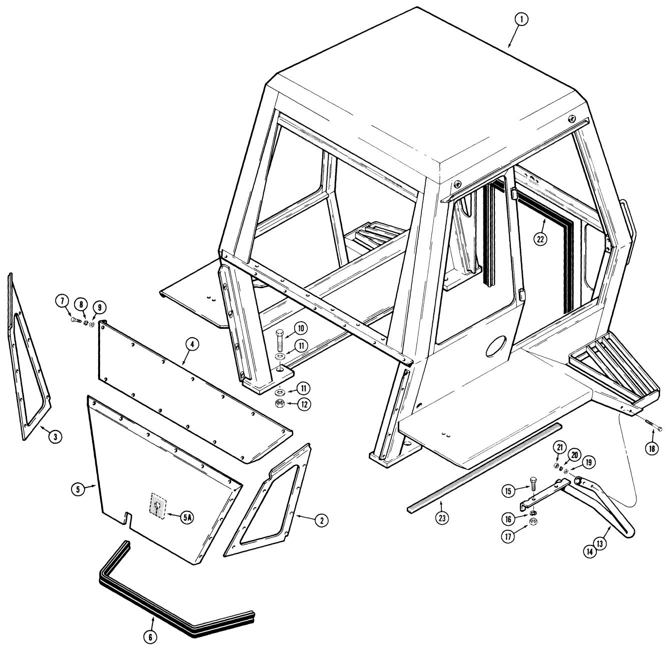
**\*OPERATOR'S CAB (CASE BUILT)
