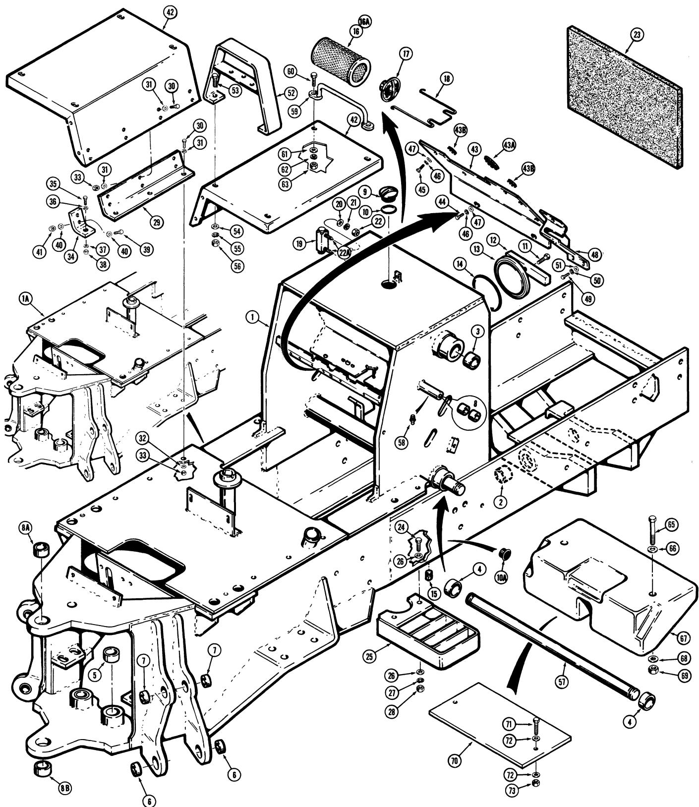
**MODEL 680E CONSTRUCTION KING LOADER BACKHOE 427****CHASSIS, FENDERS AND STEPS**
