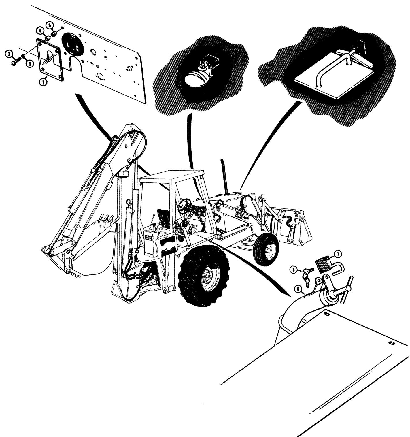
**MODEL 680E CONSTRUCTION KING LOADER BACKHOE 459****LOCKUP PARTS**
