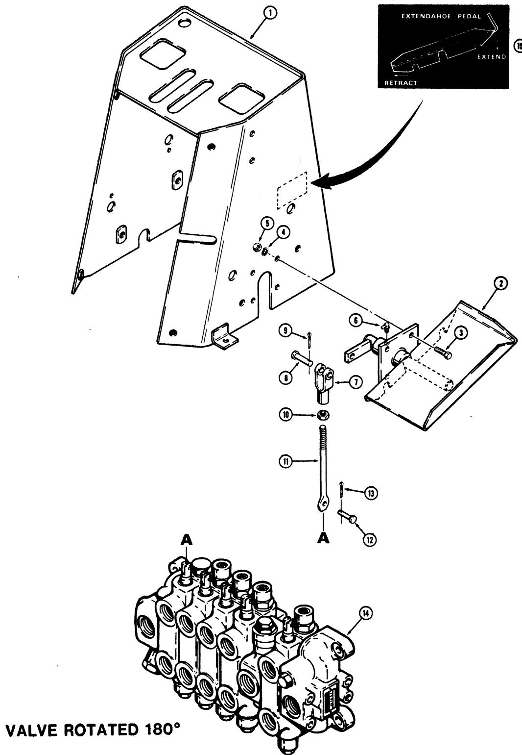
**MODEL 680E CONSTRUCTION KING LOADER BACKHOE 401****EXTENDABLE DIPPER CONTROL WITH HAND SWING MODELS**
