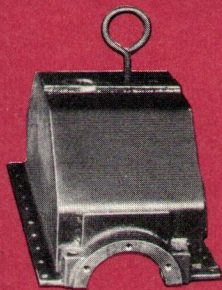
Transmission for main drum.
