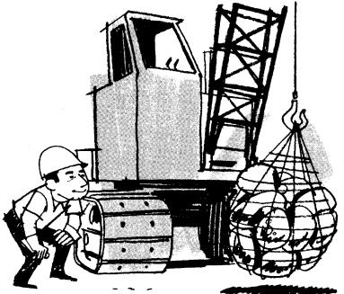
Test stability before lifting heavy loads. Check outrigger footing. Lift load slightly off the ground and stop... check machine for movement and check to be sure the brakes hold with the load elevated. Never use machine stability to determine capacity. Load capacity is determined before tipping. If there are any indications of tipping, the machine is already overloaded.
