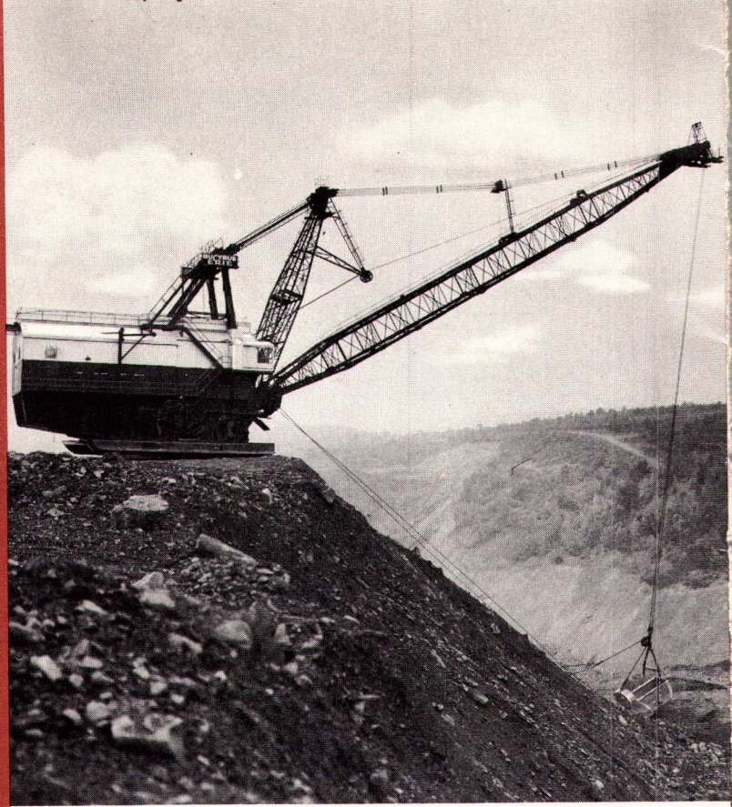
This walking dragline made coal stripping history when it went into action for Correale Construction Co. in anthracite stripping near Minersville, Pa., in 1944. Bucket size is 25 cu. yd.; boom length is 180-ft.
