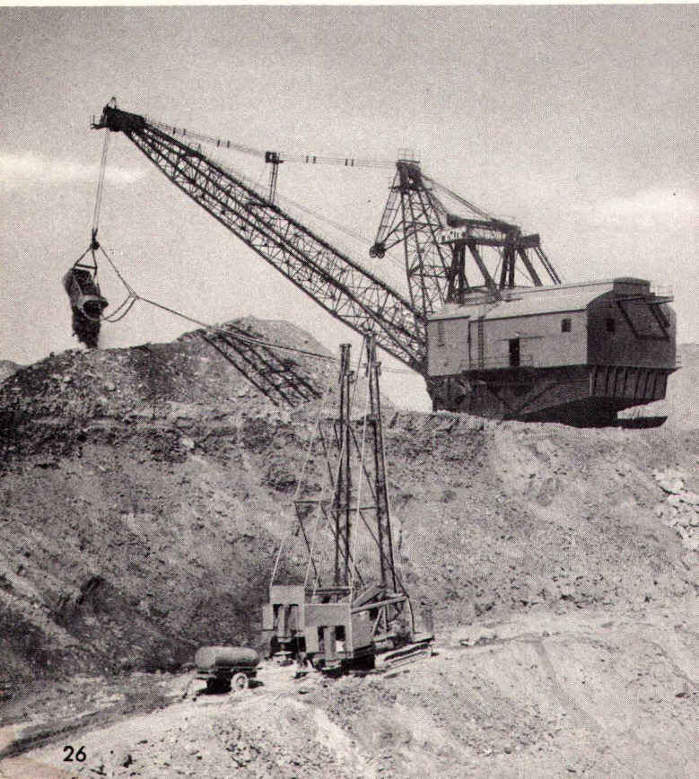
In the middle-eastern anthracite field of Pennsylvania, this walking dragline strips coal. The 25-ft. seam is covered by sandstone and clay overburden as deep as 120 ft. Owned by A. E. Dick Contracting Co., the dragline swings a 22-yd. bucket on a 200-ft. boom.
