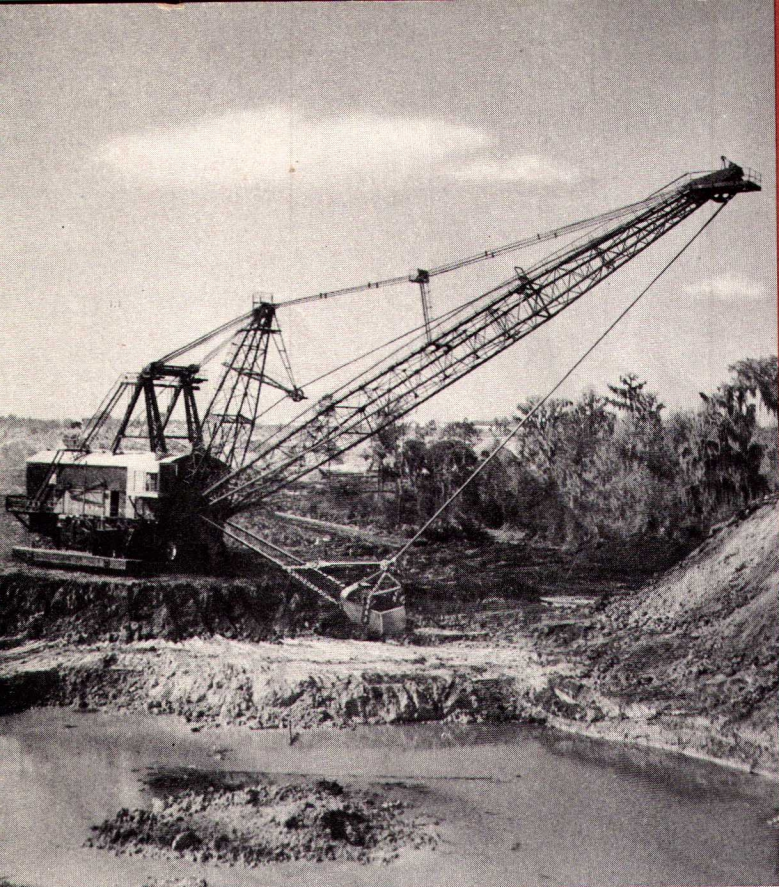
A ten-foot bed of phosphate rock plus sandy overburden averaging 22 ft. thick is excavated by this 16-yd. walking dragline at American Cyanamid Company's Saddle Creek mine in Florida. The unit is equipped with a 175 ft. boom.
