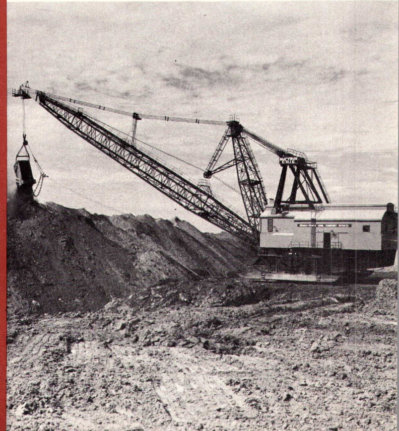
Stripping for recovery of bituminous coal at Truax-Traer Coal Company's mine near Elkhart, Ill., this 1150-B walking dragline is equipped with a 23 cu. yd. bucket. Boom length is 200 ft.
