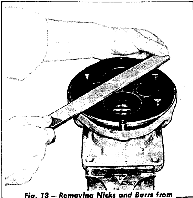
Fig. 13 – Removing Nicks and Burrs from Adapter Cover
