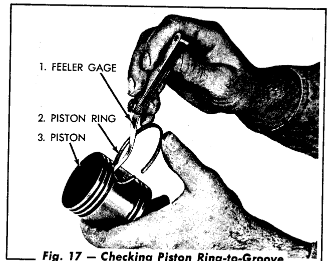
Fig. 17 — Checking Piston Ring-to-Groove Clearance
