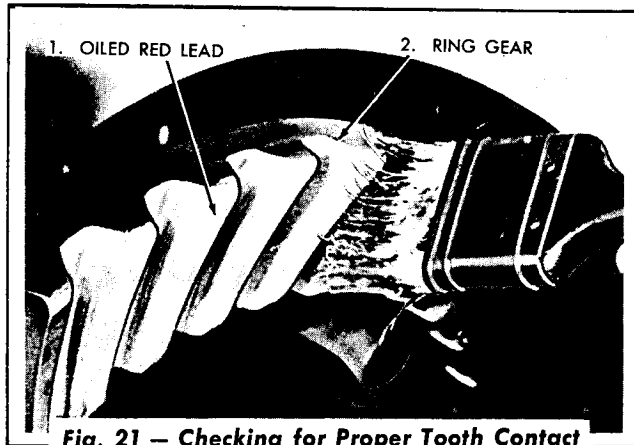
Fig. 21 — Checking for Proper Tooth Contact Between Ring Gear and Pinion Gear
