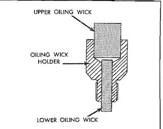
Fig. 14—Steering Clutch Throwout Sleeve Bearing Oiling Wicks and Wick Holder
