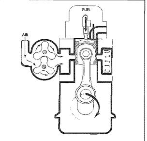
Fig. 4—Charge of Fuel Being Injected Into Combustion Chamber
