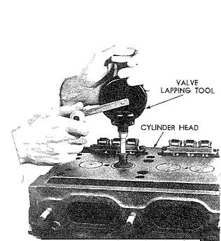
🔜 Fig. 22—Lapping Valves After Grinding 🛄
