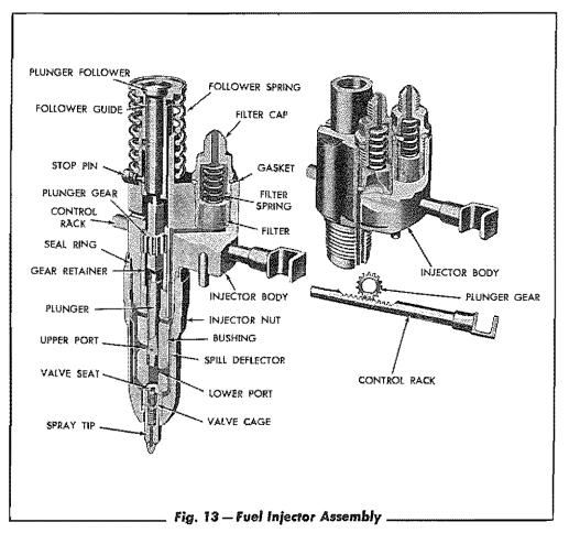
the spill deflector. The plunger operates up and down in this bushing, the bore of which is connected to the fuel supply in the annular chamber by two funnel-shaped ports.
