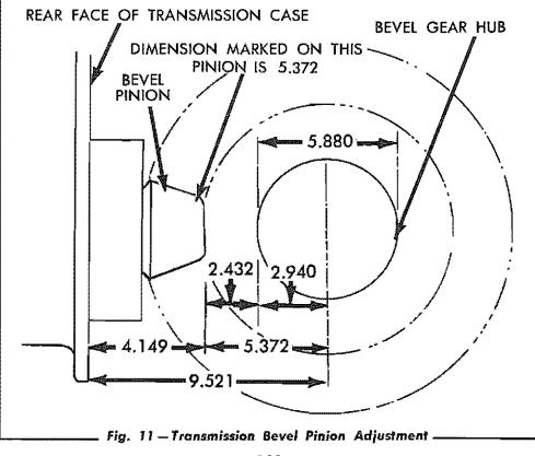
to check the tooth bearing pattern after making an adjustment (refer to Fig. 18 in this Section for proper tooth pattern).
