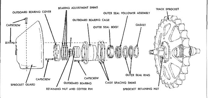
Fig. 20—Sprocket Shaft Outboard Bearing and \_ Outer Seal Details
