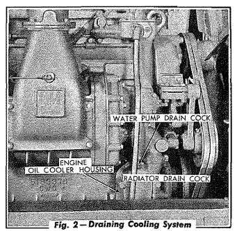
cooling system in freezing weather, make certain the coolant flows freely from all the drain cocks and that the system drains completely.
