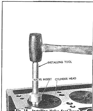
Fig. 18 – Installing Valve Seat Insert
