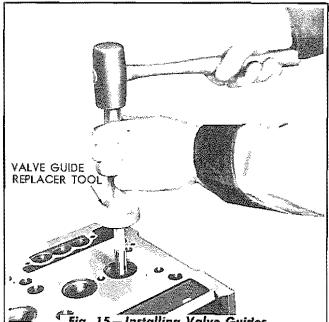
Fig. 15—Installing Valve Guides
