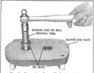
Fig. 9 – Removing Rotor Shaft Bearing from \_\_\_\_\_ End Plate
