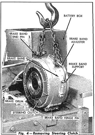
E. Disassembly of Steering Clutches
