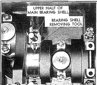
Fig. 39 – Removing Main Bearing Upper Shell
