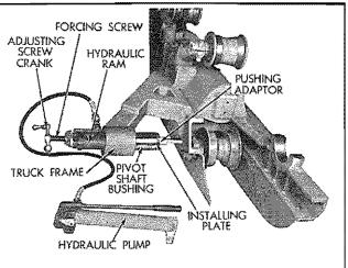
Fig. 6 — Installing Pivot Shaft Bushing .
