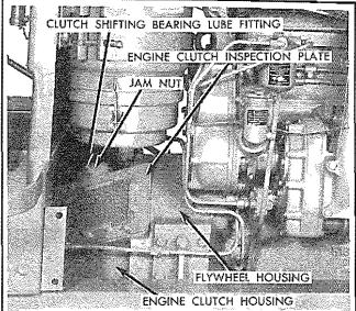
\_ Fig. 4 - Engine Clutch Inspection Plate Location
