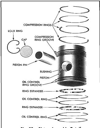
Fig. 30 — Piston Assembly Details
