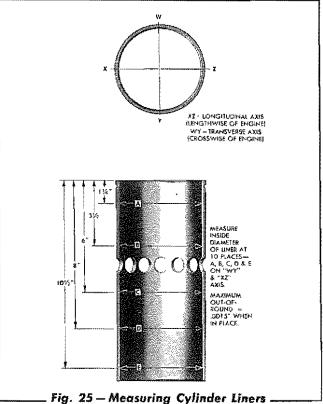
inder liners slide into the cylinder block bores freely to assure a loose fit. If the bores in the block are in a tapered or out-of-round condition, they should be honed slightly with a fixed-stone hone to remove the high spots.
