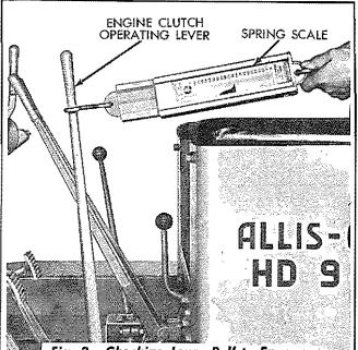
Fig. 3 – Checking Lever Pull to Engage Engine Clutch
