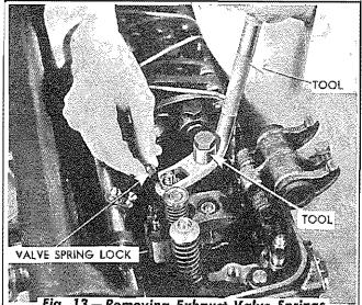
Fig. 13 – Removing Exhaust Valve Springs –
