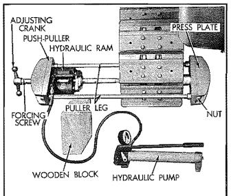
\_Fig, 6—Pressing Master Pin Into Track (Front View)
