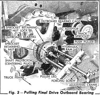
Fig. 3 — Pulling Final Drive Outboard Bearing from Track Sprocket Shaft
