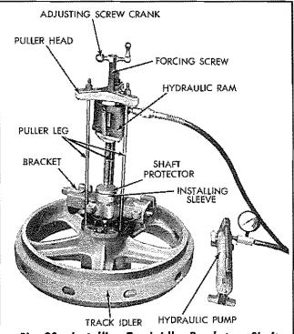
\_\_\_\_ Fig. 30—Installing Track Idler Bracket on Shaft .
