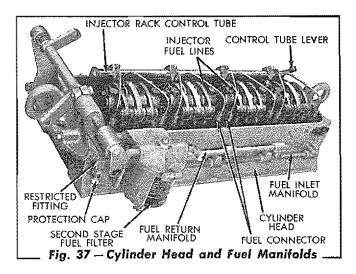
If the seating surface for the fuel connector is a trifle corroded or rough and does not make a good seal, removal of the fuel manifold and lapping of the two surfaces with a fine lapping compound may correct the leak. Clean the fuel manifold and the fuel connector thoroughly after this operation to prevent any of the lapping compound from entering the injectors. Use new copper washers under the fuel connector lock nuts when installing the manifold.
