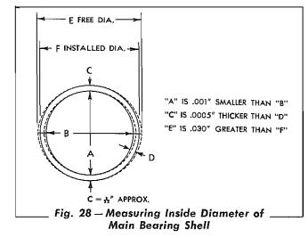
form a true circle when not installed and, when measured for inside diameter, they should be installed in the cylinder block and the bearing caps bolted tightly in place (crankshaft removed). The two (2) halves of the shells have a squeeze fit in the seat and bearing cap, and must be tight when the cap is drawn down. Tighten each bearing cap to a torque of 180 to 190 lbs. ft. using a torque wrench.
