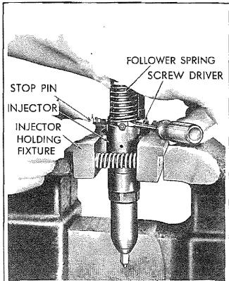
Fig. 15—Removing Stop Pin from Injector Plunger Follower
