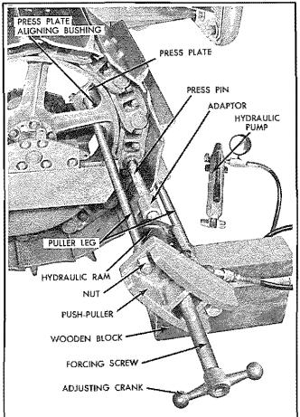
Fig. 3 – Pressing Master Pin from Track
