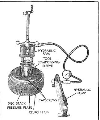
Fig. 6 – Steering Clutch Springs Compressed to \_ Remove Capscrews
