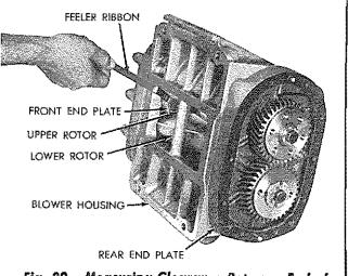
Fig. 20 — Measuring Clearance Between End of \_\_\_\_\_\_ Rotor and End Plate
