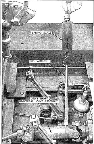
— Fig. 19 — Turning Drive Shaft Universal Joint \_\_\_\_ Assembly to Tighten Track Sprocket Retaining Nut
