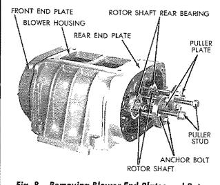
\_\_\_\_Fig. 8 — Removing Blower End Plates and Rotors \_\_\_\_
