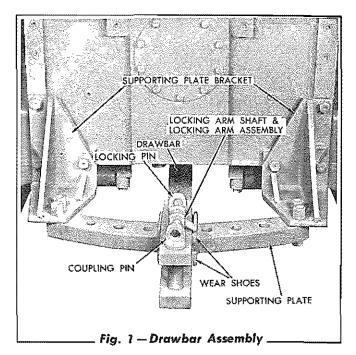
the drawbar locking pin. Both the drawbar locking pin and the coupling pin are held in position in the drawbar by the locking arm shaft and arm assembly. The bolts and capscrews attaching the hinge pin bracket and the supporting plate brackets should be checked periodically and tightened securely.
