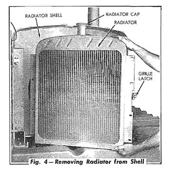
each side of the radiator to the radiator shell. Remove the radiator from the shell as shown in Fig. 4.
