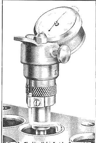
Fig. 19 - Checking Valve Seat for Concentricity
