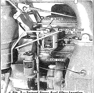
Fig. 5 — Second Stage Fuel Filter Location
