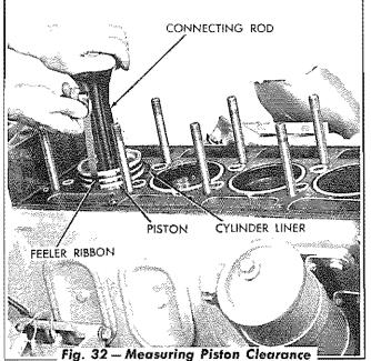
New piston rings should always be used with new pistons; furthermore, if the engine has been in service for some time, even though the same pistons are again used it is advisable to use new rings when the engine is again assembled.
