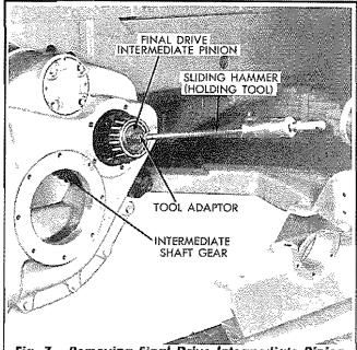
\_Fig. 7 — Removing Final Drive Intermediate Pinion \_
