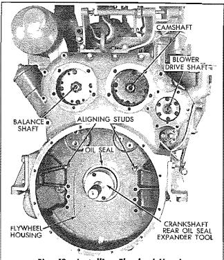
Fig. 48 — Installing Flywheel Housing
