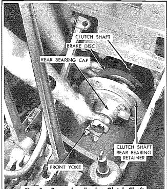
Fig. 6—Removing Engine Clutch Shaft 🔤
