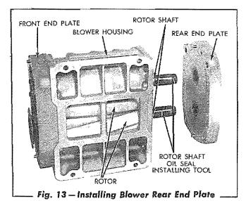
shaft facing the top of the blower housing, as explained previously in step 3, place a rotor shaft oil seal installing tool on the gear end of each rotor shaft, then install the rear end plate in the same manner as the front end plate was installed. Fasten the rear end plate to the blower housing with two (2) fillisterhead screws, using no lockwashers. The dowels in the rear end plate must project 3%" beyond the outer face of the plate. Remove the oil seal installing tools from the rotor shafts.
