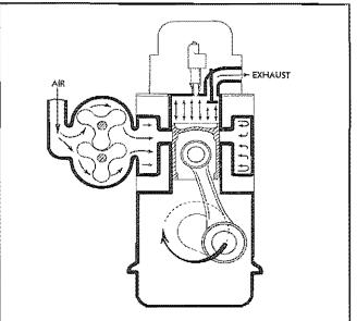
Fig. 5 — Exhaust Taking Place and Cylinders About to Be Swept with Clean Scavenging Air
