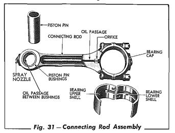
The connecting rod bearings are precision type, without shim adjustments. The upper and the lower halves of the connecting rod bearing shells are different; therefore, are not interchangeable, but are replaceable without machining.
