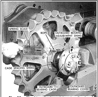
\_ Fig. 22 – Checking Outboard Bearing Pre-Load
