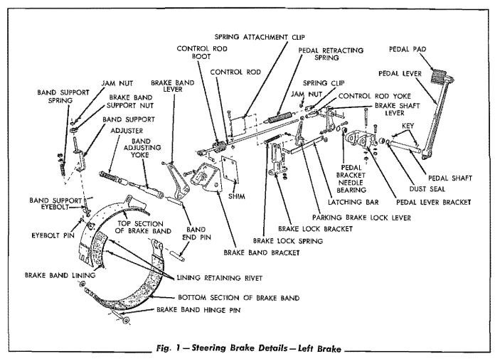
assemblies. Each brake band lever assembly is attached to both ends of the brake band. A brake pedal lever retracting spring is attached to the brake cantral rad ta return the brake pedal lever to the normal (released) position. The brake band assembly is made up of two (2) sections to permit easy removal and installatian. Each section of the brake band is serviced separately with lining attached, or the lining alone may be replaced.
