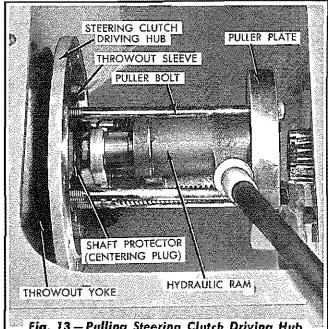
Fig. 13—Pulling Steering Clutch Driving Hub
