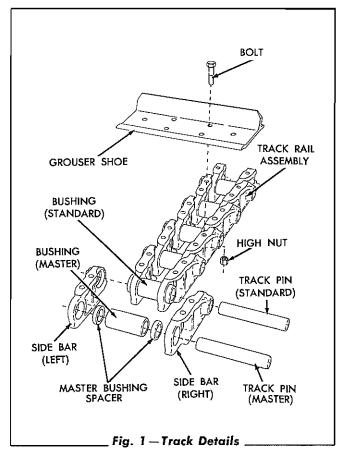
When the pins and bushings are pressed out of the track, turned 180 degrees and reinstalled, new contact surfaces are brought into play between the pin and the bushing, and between the bushing and the sprocket. If this operation is performed at the right time, track life will be prolonged.
