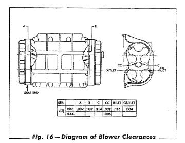
Turn the rotors, by turning the upper gear in a counter-clockwise direction, until the end of a lobe of each rotor points straight down at the gear end of the blower, as shown in Figs. 16 and 17. Insert a feeler ribbon through the opening in the cylinder block side (outlet side) of the blower housing and
