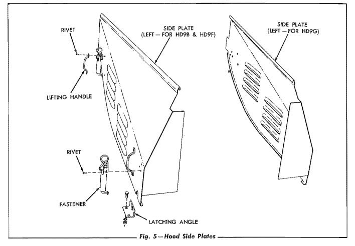
Hood side plates with louvers are available for cold weather use. The hood side plates hook to the engine hood and fasten to the front fenders
