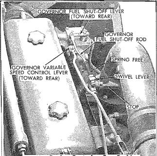
Fig. 3 – Engine Controls – Run Position shutoff lever. Hold the governor fuel shutoff lever all the way back (toward the cowl) as far as it will go and check to see if the hole in the fuel shut-off rod lines up with the hole in the governor fuel shut-off lever.
