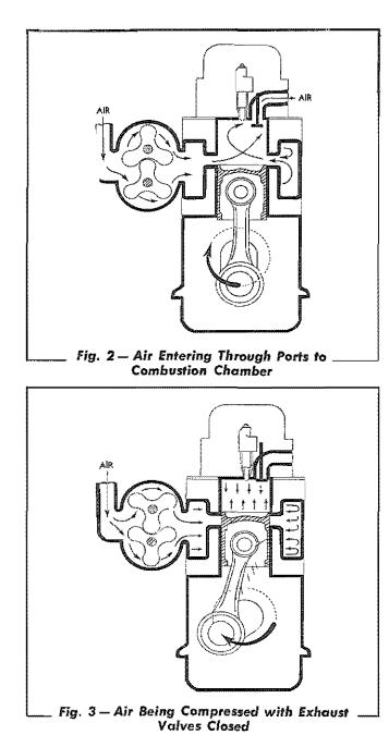
Shortly before the piston reaches its highest position, the required amount of fuel is sprayed into the combustion chamber by the unit fuel injector as shown in Fig. 4. The intense heat generated during the high compression of the air ignites the fine fuel spray immediately, and combustion continues as long as the fuel spray lasts. The resulting pressure forces the piston downward until the exhaust valves are again opened. As shown in Fig. 5, the burned gases escape into the exhaust
