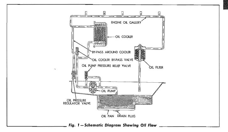
The engine lubrication system shown schematically, includes the gear driven oil pump, oil pump pressure relief valve, oil cooler, oil cooler by-pass valve, oil pressure regulator valve, oil filter, and the oil passages in the engine block and the cylinder head.
