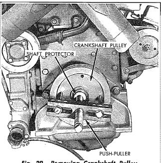
\_ Fig. 29 — Removing Crankshaft Pulley \_\_\_
