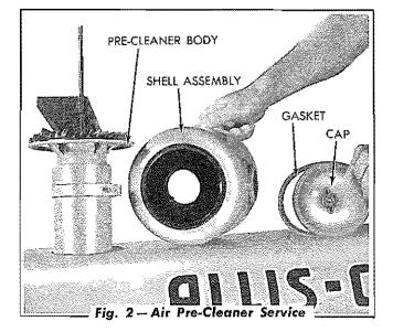
Unscrew the wing nut and remove the cap from the shell. Lift the shell from the precleaner body.
