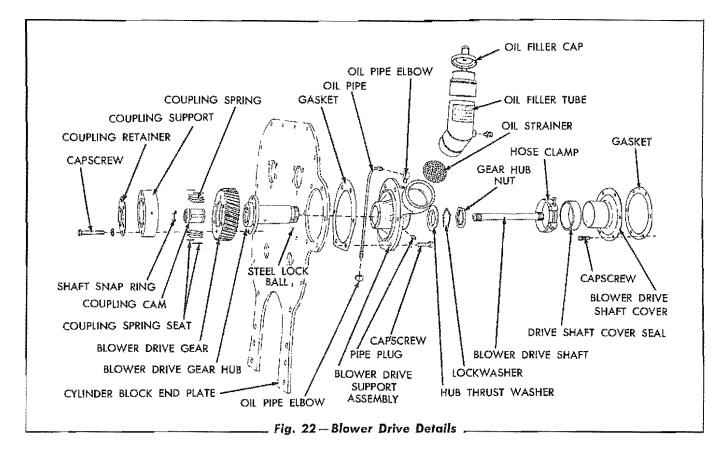
replaced, clamp the coupling support in a vise and insert the blower drive shaft into the coupling cam, then work the coupling cam out of the coupling springs. Remove the coupling springs after the coupling cam has been removed. CAUTION: Use care when removing the coupling cam so that the springs will not be lost.
