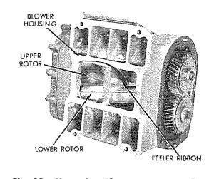
Fig. 18—Measuring Clearance Between Rotor\_ Lobes from Outlet Side
