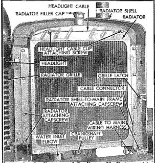
Fig. 3—Radiator and Radiator Shell Assembly
