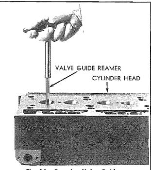
Fig. 16 - Reaming Valve Guides
