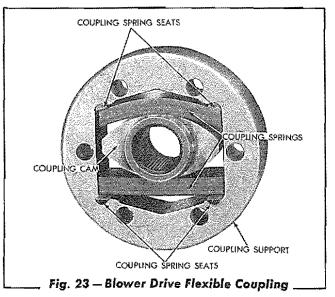
5. If the coupling springs and the coupling cam were removed from the coupling support, a small "C" clamp may be used when assembling. Lubricate the coupling springs with engine oil and divide the springs into two (2) banks of 21 leaves each. Place two (2) of the half-round coupling spring seats in position in the coupling support, then place one (1) bank of coupling springs in position
