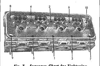
Fig. 7 — Sequence Chart for Tightening Cylinder Head Stud Nuts
