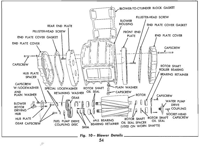
sealing lips of the seals pointing away from the inner faces of the end plates. Install each of the four (4) oil seals as follows:
