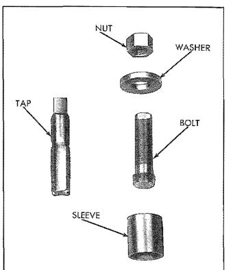
Fig. 29 – Remover Tools for Injector Copper Tube
