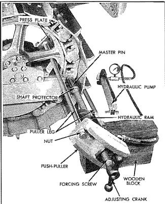
Fig. 5 – Pressing Master Pin Into Track (Side View)\_
