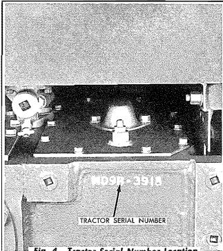
Fig. 4 – Tractor Serial Number Location —
