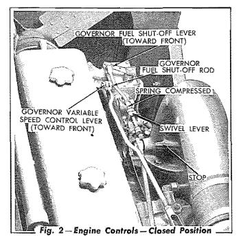
To adjust the governor fuel shut-off control, push the engine shut-off control knob forward into the running position (all the way in) and remove the pin connecting the gov-
