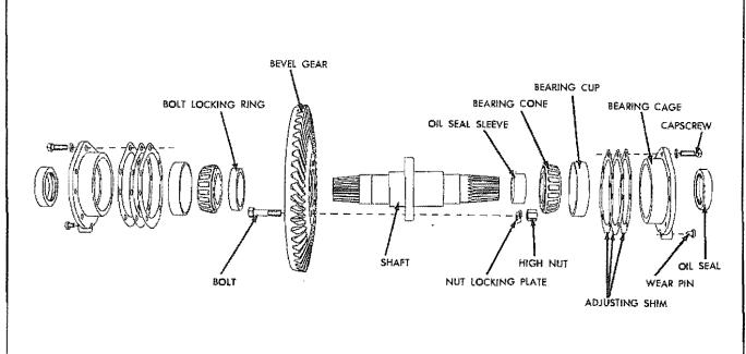
Fig. 14—Bevel Gear and Shaft Details
