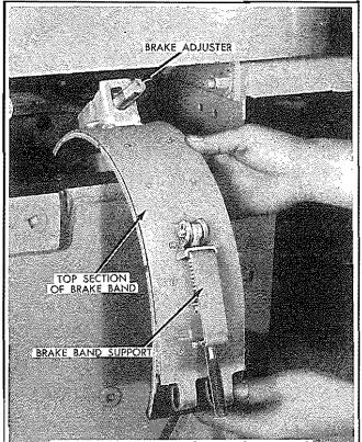
🖉 Fig. 4 — Steering Brake Band Removal 🖺
