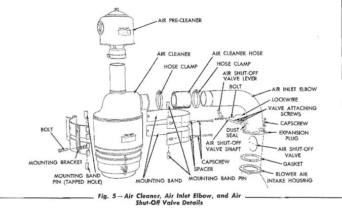
6. Clean and inspect the air shut-off valve parts for wear. The air shut-off valve shaft must be straight and not excessively worn or the valve will not seat properly in the air inlet elbow. The expansion plug in the outer side of the air inlet elbow must fit tight in its bore to prevent air being drawn past it. Always install a new shaft dust seal in the air inlet elbow when assembling. Make certain the shaft rotates freely when installed.
