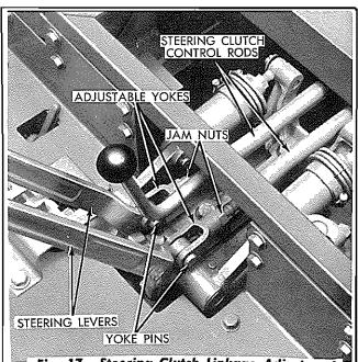
🔜 Fig. 17 – Steering Clutch Linkage Adjustment 💻
