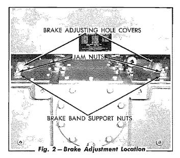
3. With the brake pedal lever free (pedal all the way back), loosen the jam nut on the brake band support, then back off the band support nut from its seat in the steering clutch compartment cover. Turn the support nut down until it contacts the seat in the cover and give the nut an additional ½ turn; this centers the brake band on the brake drum. Lock the support nut in this position with the jam nut. Install the brake adjusting hole cover.
