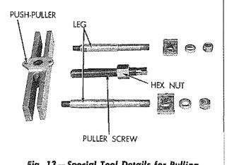
Fig. 13 — Special Tool Details for Pulling \_ Bevel Gear Shaft
