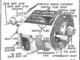
Fig. 3 — Transmission Assembly — High-Low Shift \_\_\_\_ Lever Housing and Side Cover Removed
