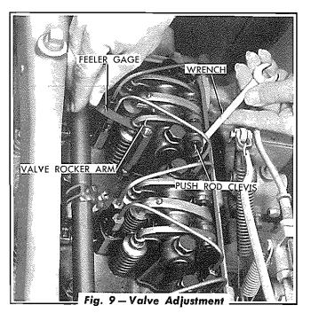
4. Crank the engine with the starter and repeat the above operation on the valves for the other cylinders. Install the rocker cover, engine hood, and the air pre-cleaner. CAUTION: If for any reason a push rod was disconnected from a rocker arm, be sure when it is reinstalled, that the upper end of the push rod is flush with the inside of the clevis yoke before cranking the engine. If it
