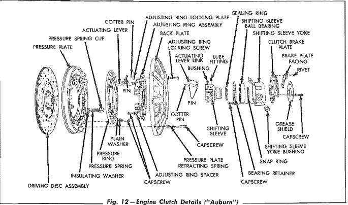
work loose. When installing the pins used to connect the actuating lever links, install the pins so that the head of each pin is to the left, with the pin located at the top of the clutch and when viewed from the rear. When installing the self locking nuts on the retracting spring screws, tighten the nuts against the retracting springs so that the assembled length of each spring is 1-3/16" (measured to bottom of recess in clutch back
