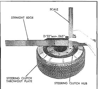
\_ Fig. 12—Measuring Distance Between Steering \_ Clutch Hub and Throwout Plate
