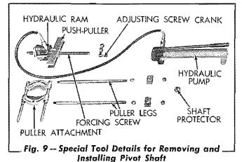
onto the pivot shaft, care MUST be used to prevent damaging the lubricating wick holder. Misalignment of the truck frame and abnormal wear of the pivot shaft and bushing will result from a damaged lubricating wick assembly.
