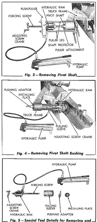
Installing Pivot Shaft Bushing
