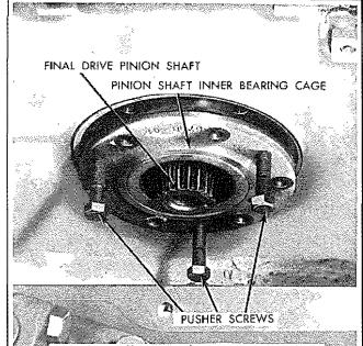
Fig. 9 – Pulling Final Drive Pinion Shaft – Inner Bearing Cage
