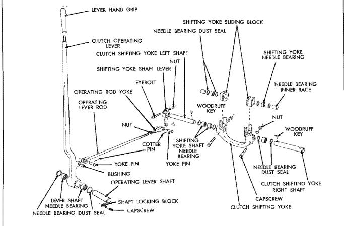
Fig. 9 – Engine Clutch Shifting Yoke Details –
