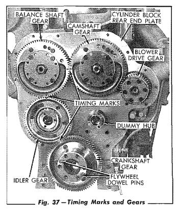
(opposite the idler gear hub location). The idler gear bearing is lubricated through a hollow dowel, communicating with the left rear vertical oil passage in the cylinder block. The blower drive gear, in mesh with the camshaft gear, transmits power to drive the blower, governor, water pump, and the fuel pump.
