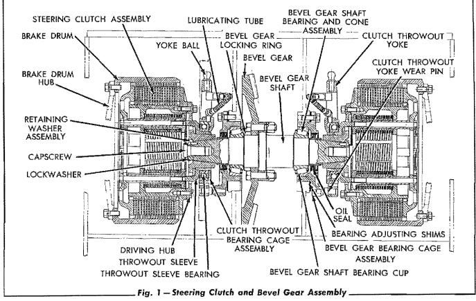
the steel discs and friction discs of the clutch to separate.
