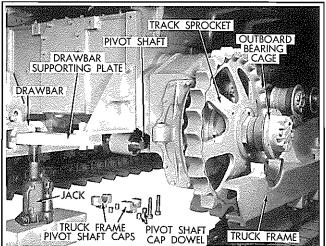
Fig. 2 — Truck Frame Assembly Ready for Removal
