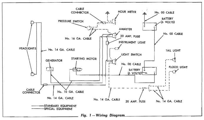
Heavy cables connect the batteries and the starter, 10 gage cables connect the ammeter and generator, and 14 gage cables connect the remaining units. A 20-ampere fuse, connected into the cable extending from the ammeter to the light switch, prevents burning out of the lights in the event of a short-circuit. An additional fuse is provided in the electrical cable, near the rear of the tractor, for protection of special lighting equipment.
