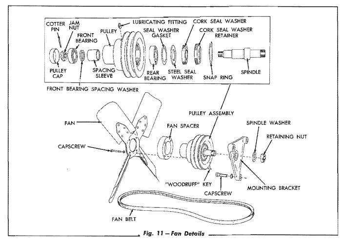
dle in a press, and press the spindle out of the bearings.
