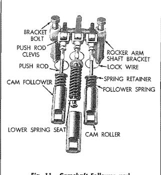
Fig. 11—Camshaft Follower and . Push Rod Assembly
