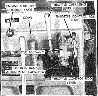
Fig. 1—Throttle Assembly and Engine Shut-Off Control Knob Location
