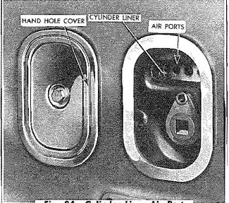
Fig. 24 - Cylinder Liner Air Ports
