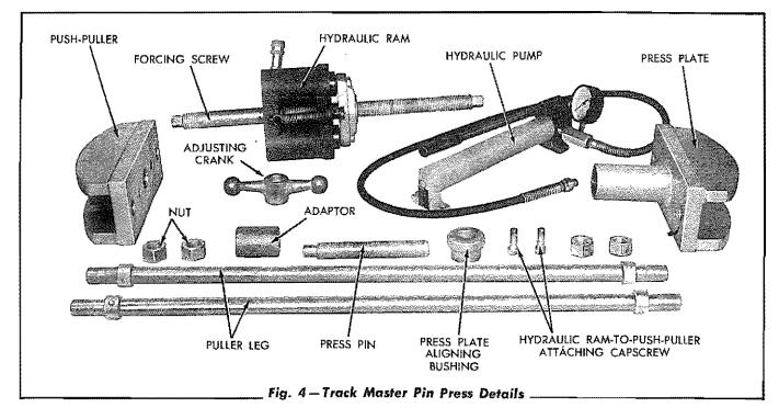
sure from the hydraulic pump and at the same time, turn the adjusting crank to move the forcing screw forward until the pistons are fully retracted into the ram cylinders. Close the actuating valve on the hydraulic pump and continue this operation until the master pin is pressed out of the track rail assembly. Remove the press assembly.
