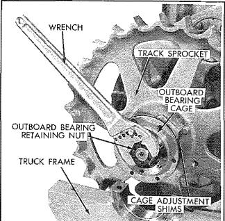
Fig. 2 – Removing Final Drive Outboard Bearing Retaining Nut
