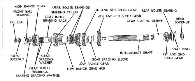
Fig. 7 – Transmission Intermediate Shaft Details\_
