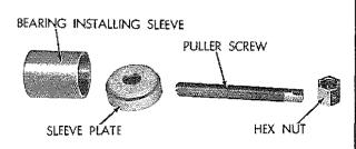
, Fig. 16—Special Tool Details for Installing Bevel \_ Gear Shaft Bearing Cone
