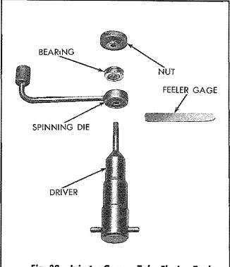
Fig. 32 — Injector Copper Tube Flaring Tool .\_\_
