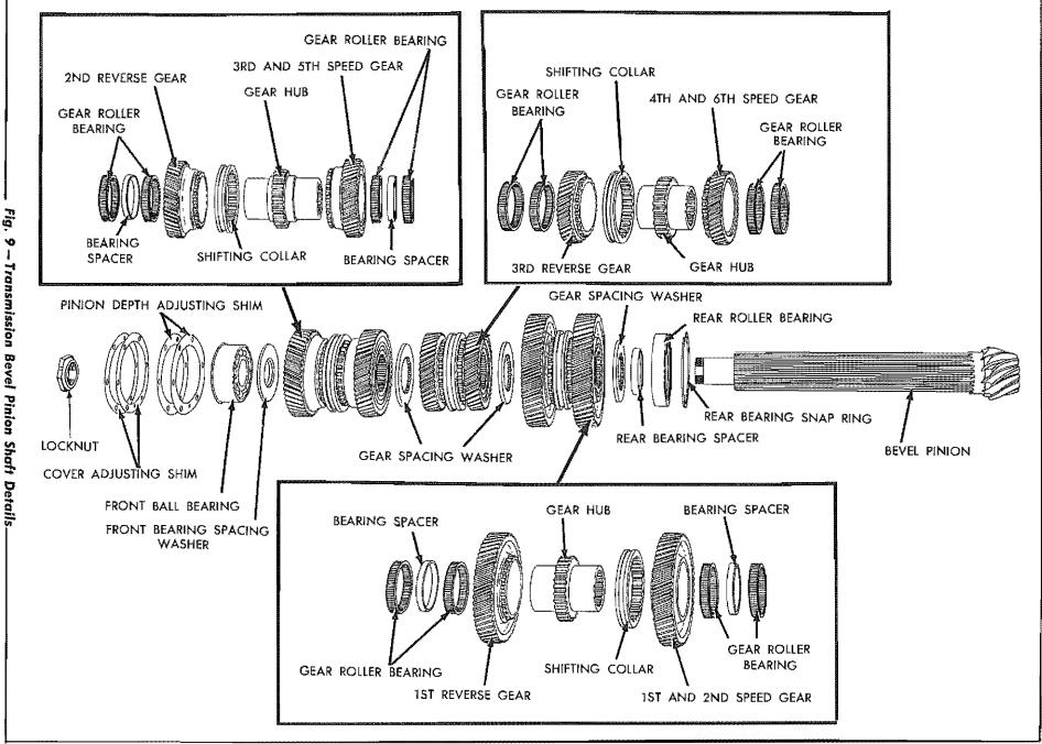
v ł Transmission **Bevel Pinion Shaft Detail**
