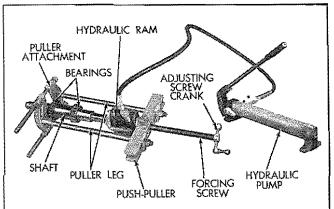
\_Fig. 15—Installing Bearings on Truck Wheel Shaft\_
