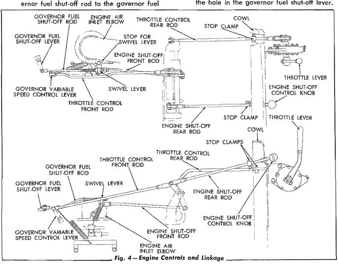
If not, loosen the capscrew clamping the governor fuel shut-off lever to the shaft, and move the position of the lever on the shaft so that the holes line up when the lever is held all the way back. Tighten the capscrew used to clamp the fuel shut-off lever to the shaft, then install the control rod pin and cotter pin.
