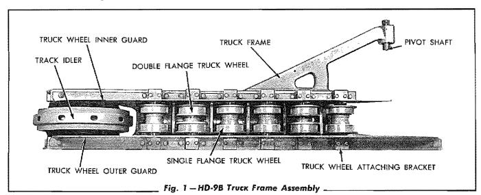
guard equipment is attached to the truck frames by capscrews and is readily removable.
