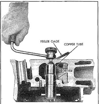
\_ Fig. 33—Flaring End of Injector Copper Tube \_
