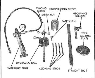
– Fig. 7 – Special Tool Details for Disassembly and J Assembly of Steering Clutch
