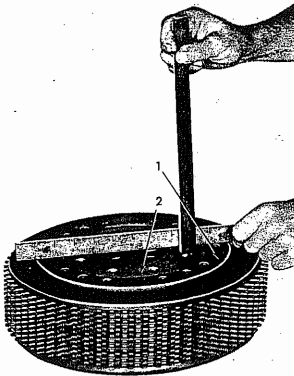
Fig. 16 -- Measuring Distance From Clutch Hub To Throwout Plate (HD7G Shown, HD6, 11 Similar) (T-36845)
