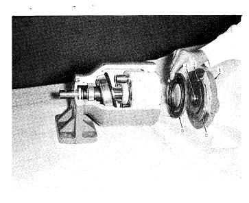
Remove rotor and pistons.
