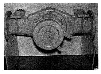
Remove pinion shaft nut and washer.
